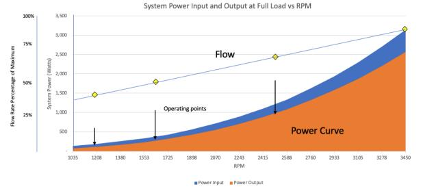
3.45HP variable speed pool pump motor and control power required at three pool operating speeds. Input power ranges from over 3000 watts at 3450 rpm to a low of less than 150 at 1200 rpm.
