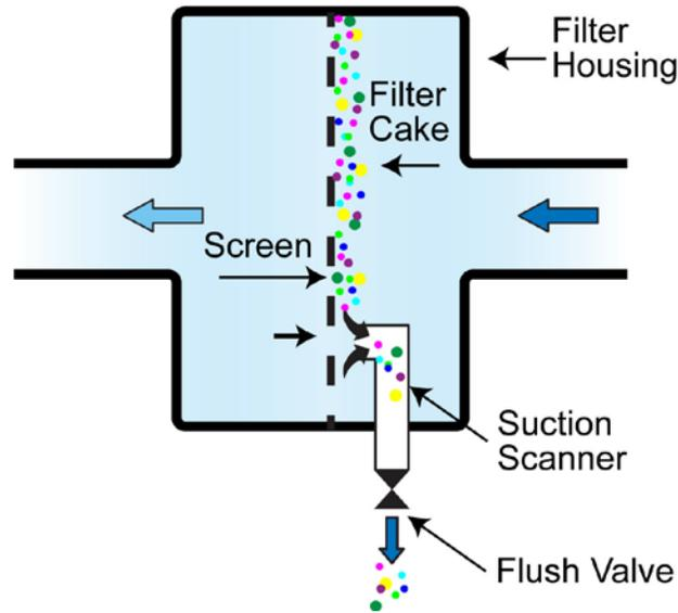
**Figure 2.2. Automatic Screen Filter Schematic.**
