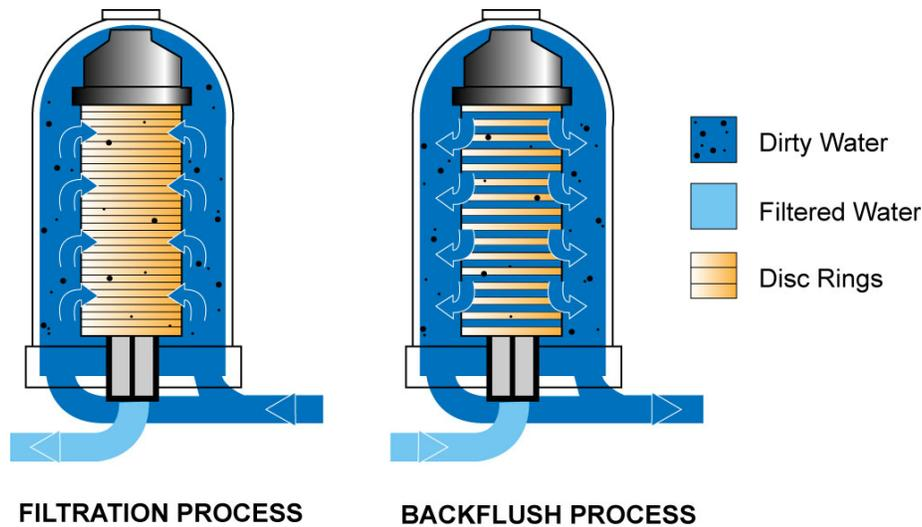
**Figure 2.3. Plastic Disc Filters.**
