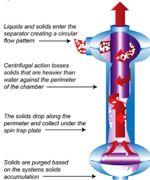
**Figure 2.1. Centrifugal Separator Schematic.**
