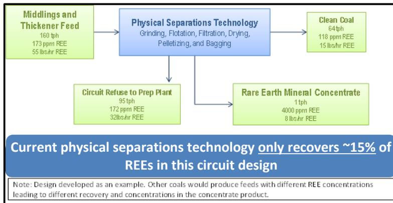
Figure 10. Rougher Circuit
