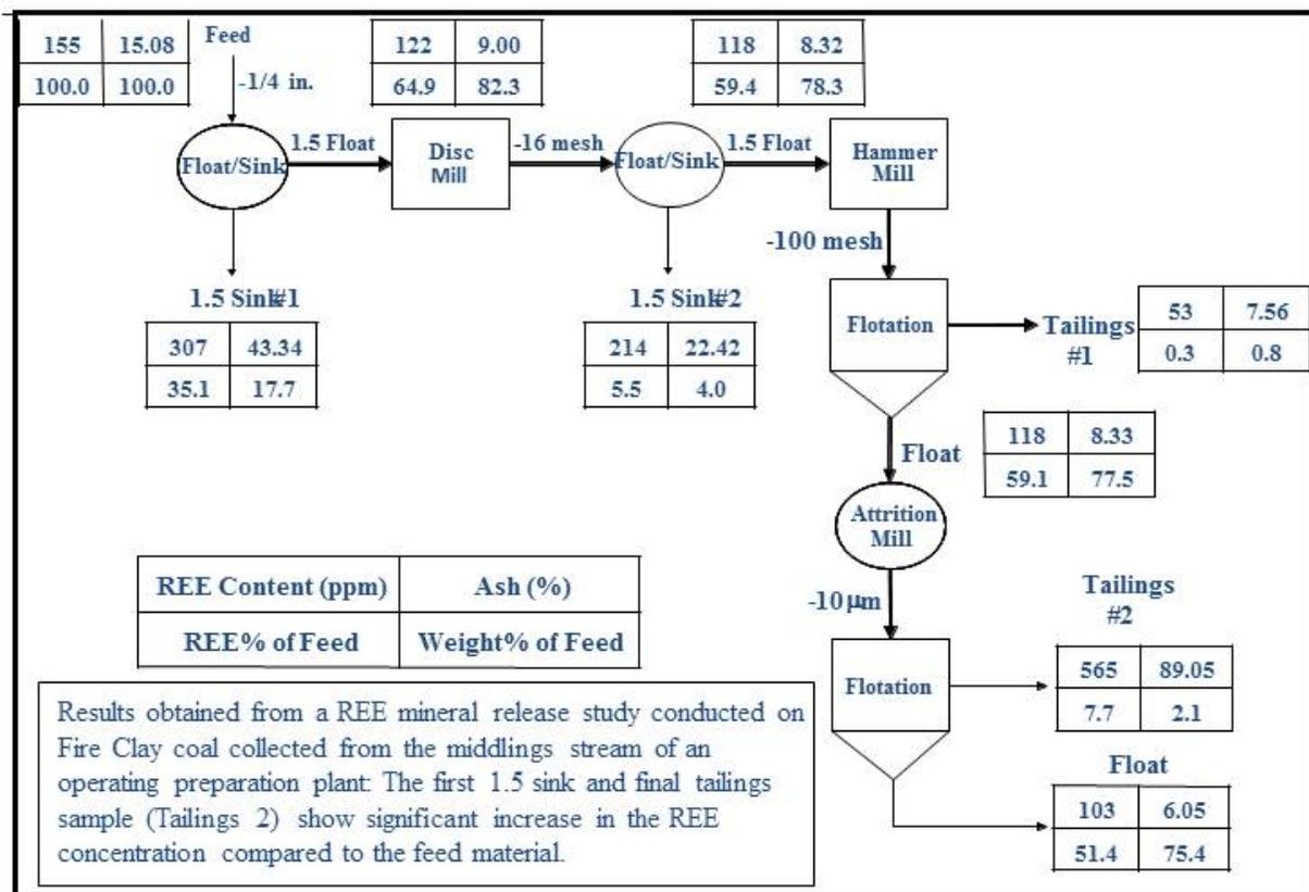
Figure 7. Mineral Release Test, Fire Clay Coal
