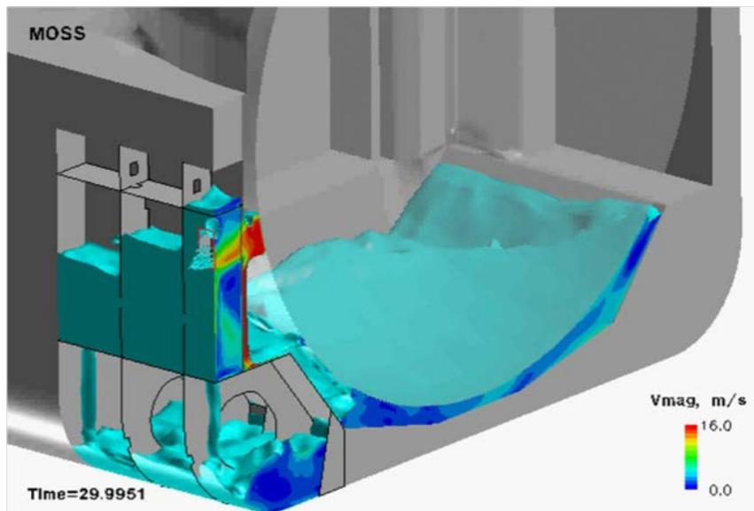
**Figure 4. Membrane LNG vessel spill and internal flow analysis examples.**
