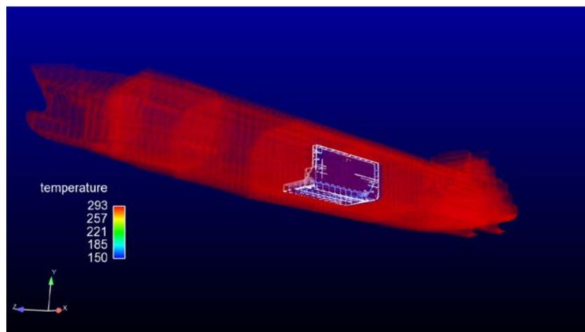
The white colored elements indicate the cryogenic fractures calculated after reaching the critical strain criterion during cooling. The transparent view shows both the cracking in the outer hull and inner hull surrounding the cargo tank. Here, the extent of the damage to vessel structure surrounding the breached cargo tank can be seen. The analysis predicts cracking will occur throughout the entire cooled region, which reflects those portions of the vessel that were exposed to LNG flow.
