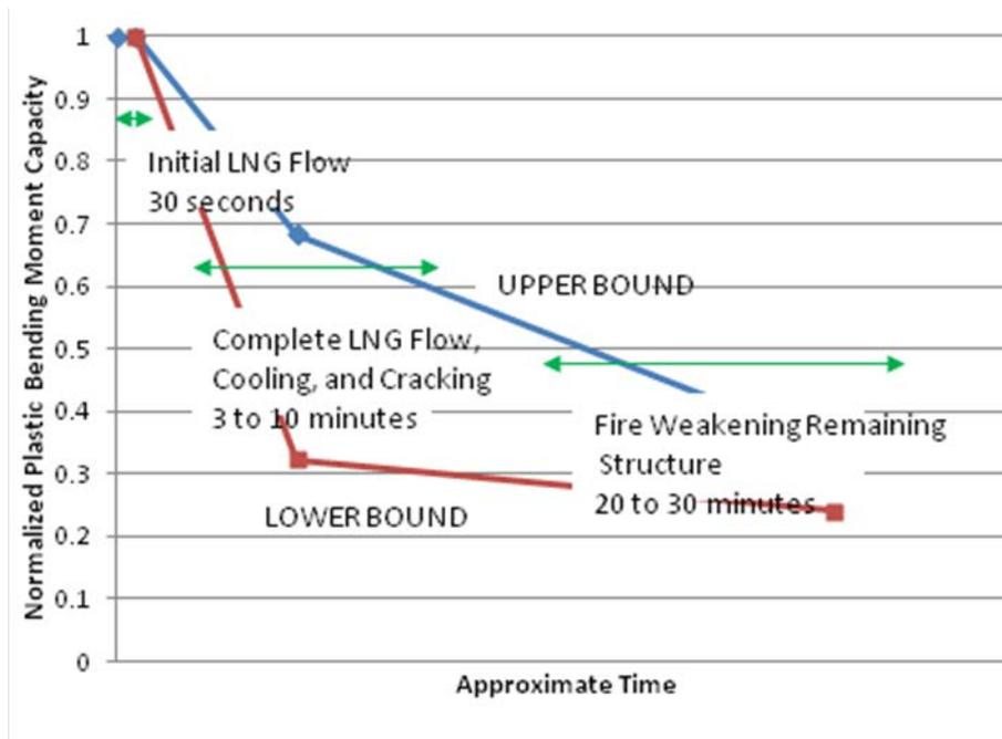
The plastic bending moment capacity is defined as the bending moment that would lead to the entire cross-section of the vessel yielding and creating essentially a plastic *hinge*. The plastic bending moment capacity is often used in extreme event risk analyses to evaluate the level of residual structural capacity following an extreme event.
