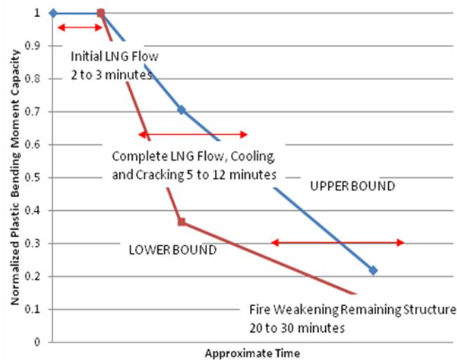
The cryogenic damage causes an approximate 40 to 70 percent reduction within 5 to 12 minutes (including several minutes to account for the slower flow calculated for the Membrane vessel design) with the fire causing a 80 to 90 percent total reduction in the plastic bending moment capacity between 20 and 30 minutes. The fire has a more significant effect on the Membrane vessel section modulus due to the greater amount of structural cross-section that is exposed to the fire.
