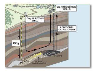
EOR is a way to recover additional domestic oil resources from older fields and permanently store carbon dioxide underground. (Illustration: Clean Air Task Force, available at: http://www.coaltransition.org/pages/carbon\_storage/30.php.)
