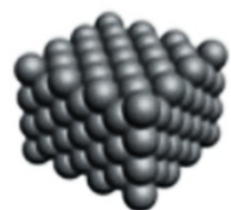
3D opal template (200 nm PMMA colloids on substrate)
