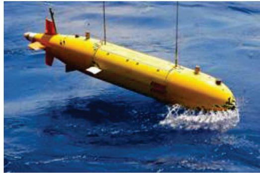
**Figure 4.10.** (a) Novel remote sensing under water with autonomous underwater vehicle and (b) airborne electromagnetic sounding using a torus helium balloon. | (a) image from CTEMM-CCS website (<http://www.stemm-ccs.eu/work-packages>). Used by permission of Doug Connelly, National Oceanography Centre, UK.
