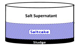
The sludge portion along with high activity constituents from the salt stream are being transferred to the on-site DWPF for vitrification into borosilicate glass to immobilize radioactive constituents.
