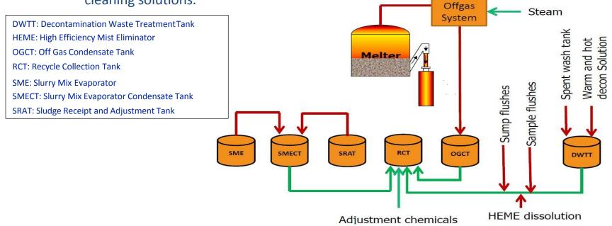
Currently, the DWPF recycle wastewater is returned to Tank 22 for volume reduction by evaporation (2H evaporator), or is beneficially reused in saltcake dissolution or sludge washing.
