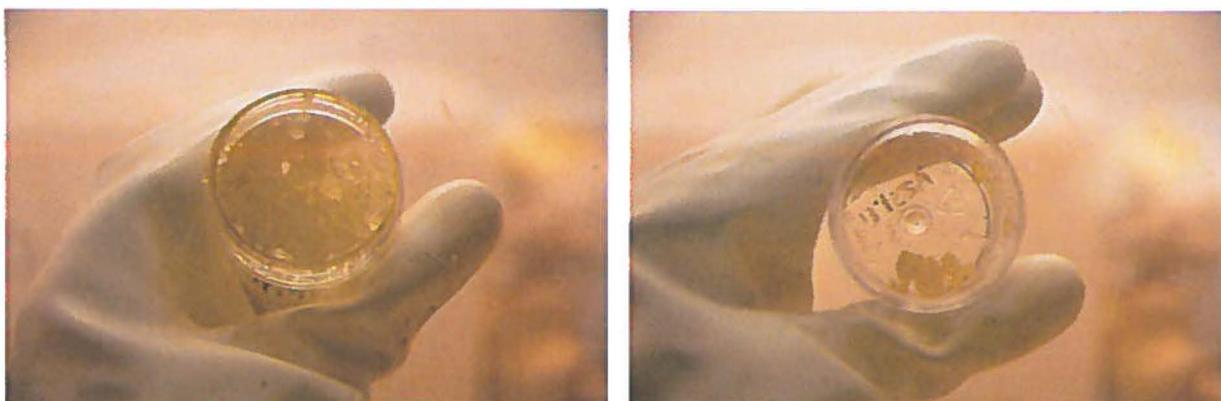
*Figure 1: Evaporator bottoms—hydrated nitrate salts of sodium, potassium, calcium, magnesium, and aluminum*
