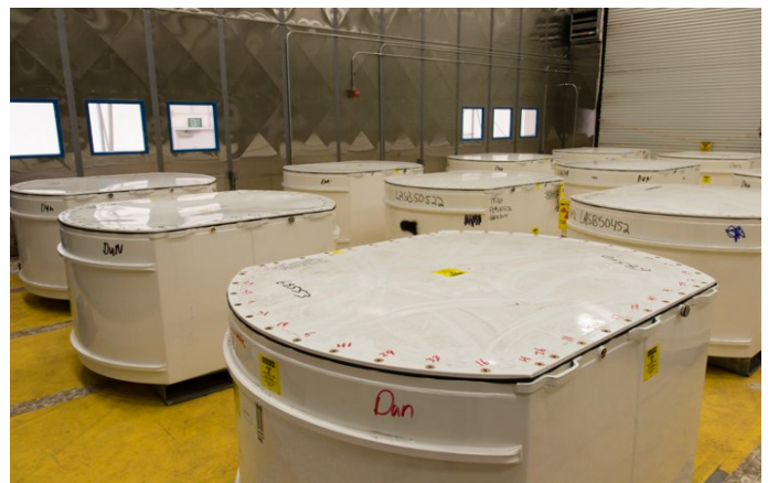
RNS drums are packed inside standard waste boxes inside the PermaCon.
