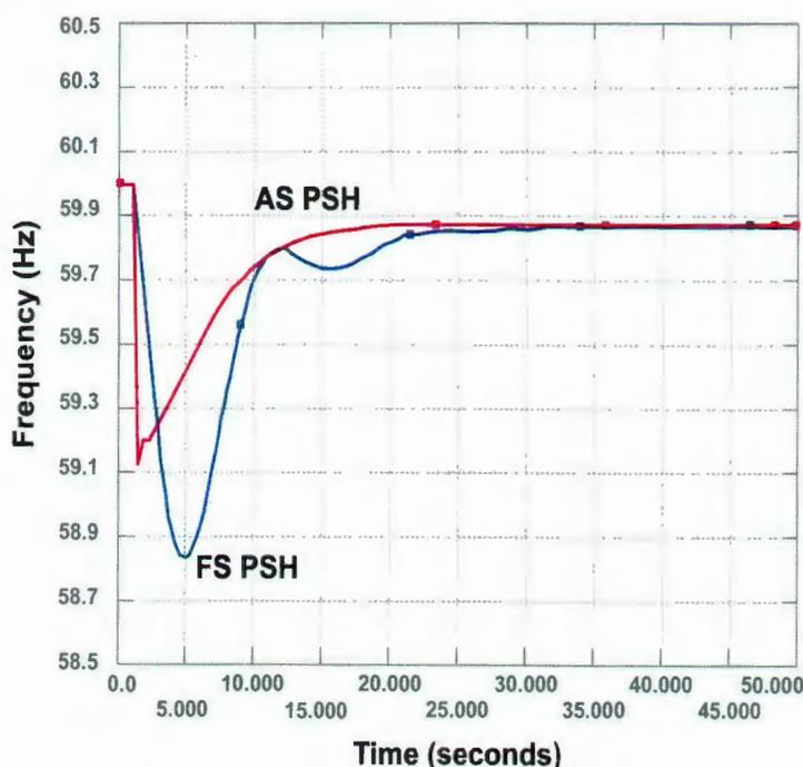
Figure 4. System Frequency with FS and AS PSH after a Gas Turbine Outage (Source: Koritarov et al. 2014<sup>9</sup>).
