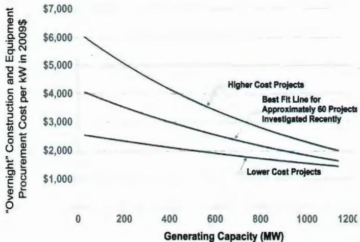
Figure 7. Estimated Construction Costs of New PSH (Source: USACE 2009<sup>6</sup>).
