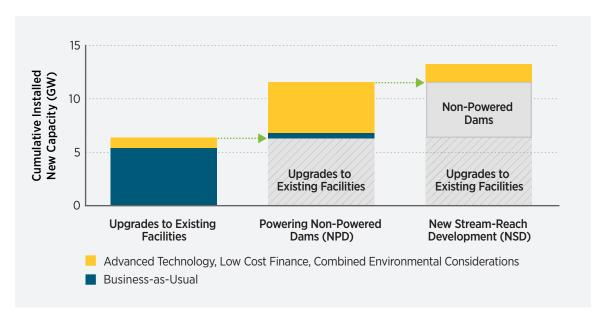
Figure ES-6. ReEDS modeled cumulative 2050 deployment of new hydropower generation capacity by resource category (GW)
