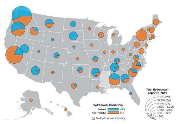
Figure ES-1. Existing hydropower generation capacity in the United States (79.6 GW)
