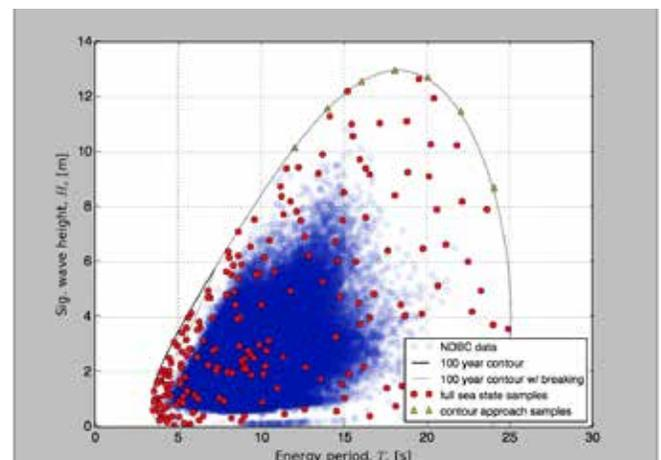
Analysis of National Data Buoy Center (NDBC) wave data to give 100-year return contour and sampling of sea states for survival analysis performed with [WEC Design Response Toolbox \(WDRT\)](#).
