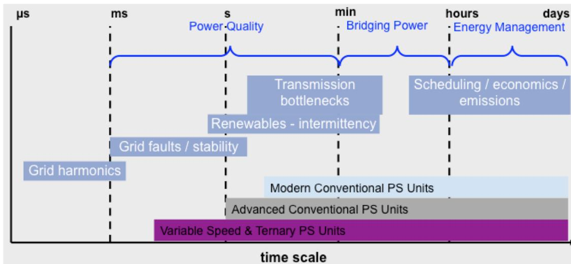
Figure 2-9 Timeframes for modern advanced PS unit regulation
