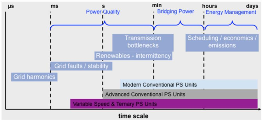
**Figure 3-6 Timeframes for advanced pumped storage unit regulation**
