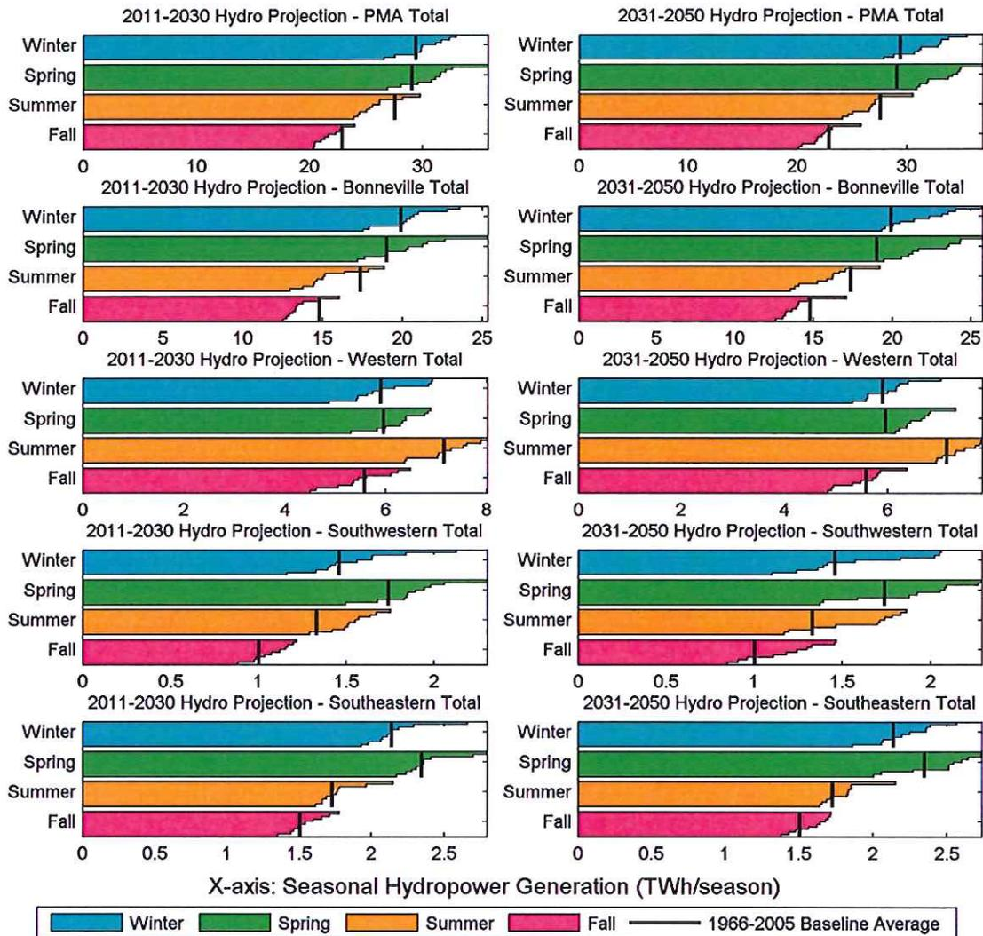
**Figure 5. Summary of the seasonal hydropower projection in the near-term (2011–2030) and midterm (2031–2050) future periods for each PMA. Each bar consists of 10 smaller bars for each downscaled climate model (sorted descending from top to bottom). The multimodel baseline (1966–2005) average is marked in the bold line for comparison.**
