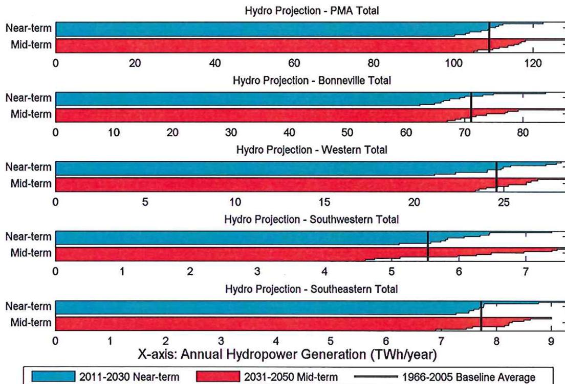
**Figure 4. Summary of annual hydropower projection in the near-term (2011–2030) and midterm (2031–2050) future periods for each PMA. Each bar consists of ten smaller bars for each downscaled climate model (sorted descending from top to bottom). The multimodel baseline (1966–2005) average is marked in a bold black vertical line for comparison.**
