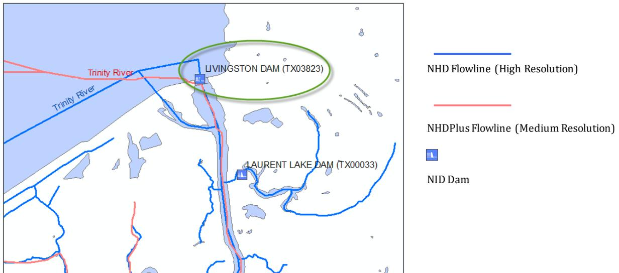
**Figure 5. Illustration of linkage between NID and NHDPlus** – In NID, Livingston Dam is linked to an NHDPlus flowline (in red color), which represents the Trinity River. The accumulative drainage area for this NHDPlus flowline is 16,572 square miles, which will be used as the dam’s drainage area.
