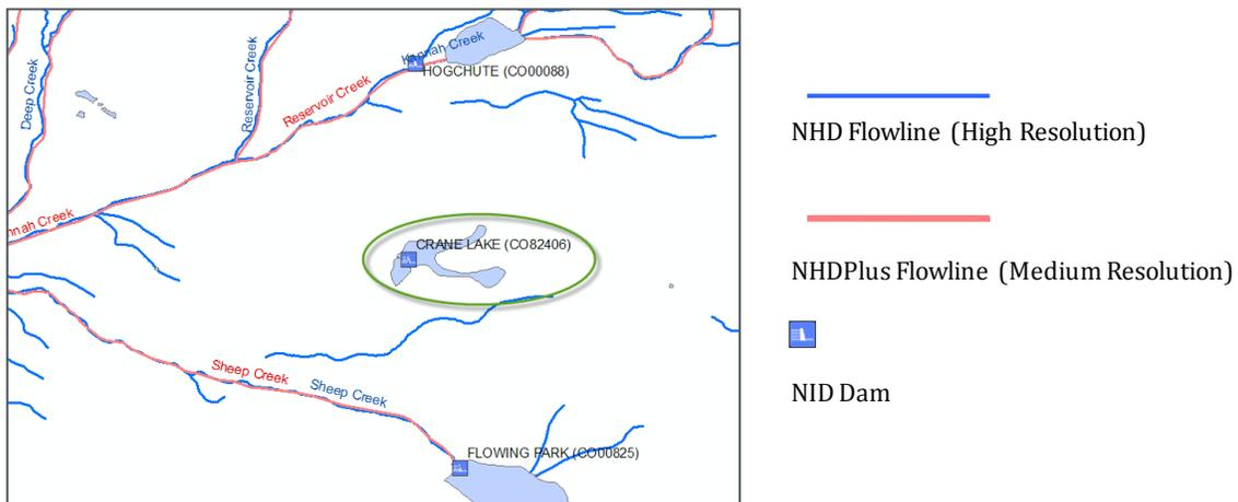
**Figure 4. Illustration of the second criterion for selecting DWNS** – In this example, because the dam “Crane Lake” is not close to any NHD flowline or NHDPlus flowline, it cannot be linked to any stream and is designated as located on segment with negligible streamflow.
