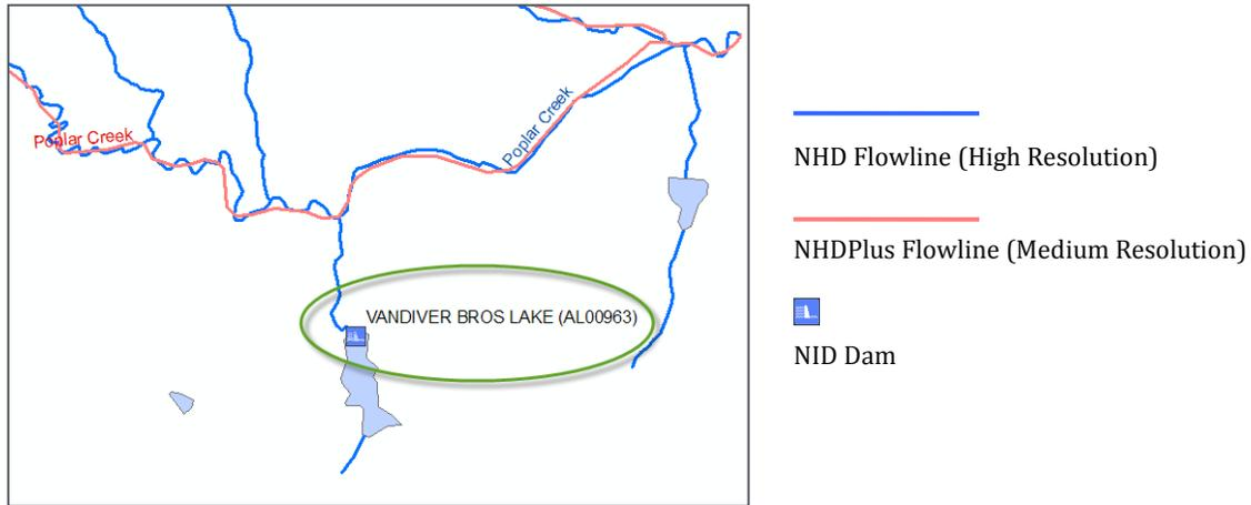
**Figure 3. Illustration of the first criterion classification of DWNS** – In this example, because the dam “Vandiver Bros Lake” is close to NHD flowline but far from NHDPlus flowline, it is designated as located on segment with negligible streamflow.
