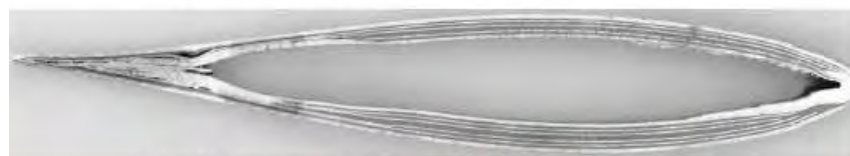
Figure 3 – Cross-section of the ORPC-supplied foil showing the laminate layup.
