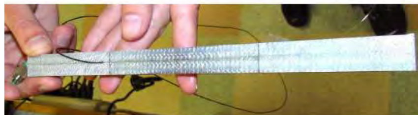
Figure 4 – Test specimen with a mounted MOI bare FBG sensor.
