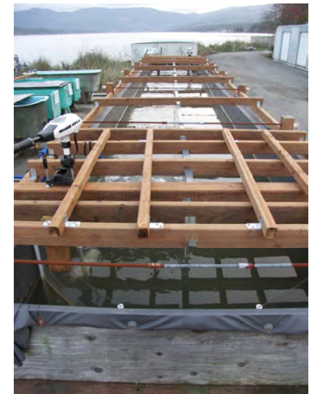
View inside the high velocity current tank. The tank is 36' long, 5' wide, and approx 30" deep.
