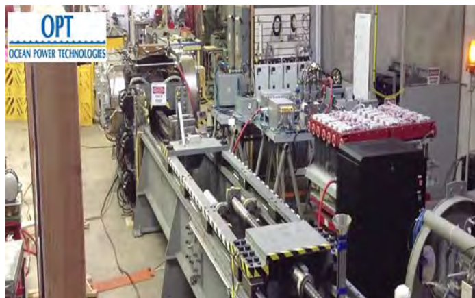
PTO endurance test setup at OPT
