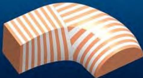
Reusable half-section molds made of Styrofoam and wood are used to fabricate Carbon composite moldings of the Venturi turbine, discharge elbow, submarine enclosure, and impeller nose cone
