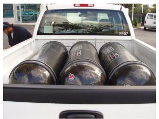
Figure 1. Dynetek hydrogen fuel tanks in the bed of the pickup.
