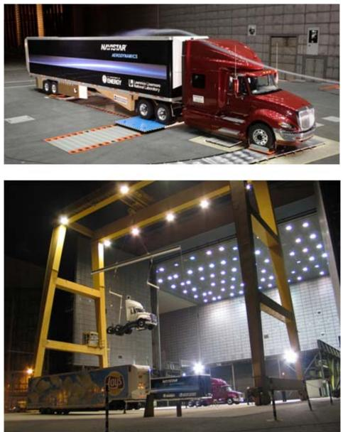
Figure 1. Top) Long-sleeper tractor and 53' straight-frame trailer in the 80'x120' NASA Ames wind tunnel. Bottom) Day-cab tractor being lifted into the wind tunnel test section. The drop-frame trailer, straight-frame trailer, and long-sleeper tractor are visible at the bottom of the photo.
