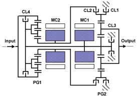
Figure 4. Schematic of the two-mode EVT with FGs
