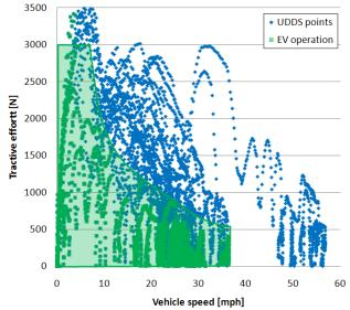
Figure 9. Electric-only Operation Area Overlaid with Urban Cycle Operating Points
