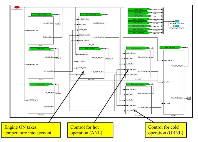
Figure 2: Reconfiguration of vehicle powertrain controller (supervisory controller) for integration of hot and cold strategy management.
