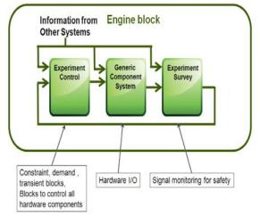
Figure 3. Engine in the loop configuration in Autonomie for easy migration from simulation to engine in the loop testing.
