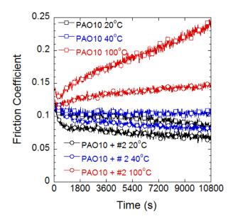
Figure 5: Friction test results for PAO10 and PAO10 containing 3 wt% BN/surfactant at 20°C, 40°C, and 100°C.
