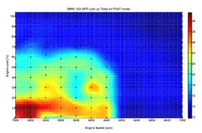
Figure 6. Steady state Air Fuel Ratio as a function of engine speed and load.
