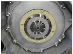
Figure 8. Engine Torque Sensor Mounted to Transmission Input
