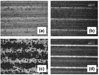
Figure 8: Microscope images of all samples tested using fully formulated 10W30 oil at 120°C using a load of 250 N: (a) uncoated, (b) DLC, (c) graphite-resin, and (d) Ni-PTFE
