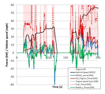
Figure 8. Fusion Operation on a Hot-start UDDS
