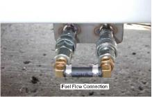
Figure 7. Fuel Measurement Connection
