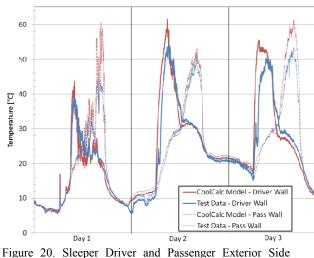
Figure 20. Sleeper Driver and Passenger Exterior Side Walls
