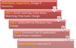
Figure 1. Test flow for the Validation Stage
