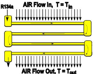
Figure 10. Current Condenser/Evaporator Configuration (Each Layer of Tubes is Represented with one Tube only in this Sketch)
