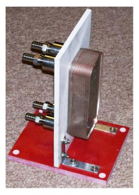
Figure 4. Heat Exchanger (Cooler) Component
