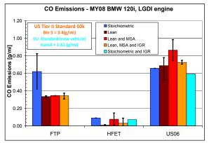
Figure 3. CO emissions as a Function of Vehicle Mode and Drive Cycle.
