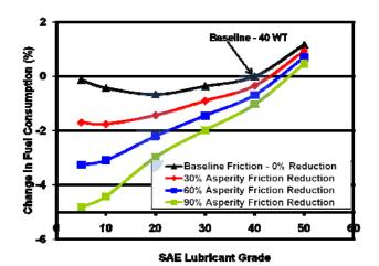
Figure 1.: Predicted change in fuel economy as a function of engine lubricant viscosity and boundary friction for an on-road driving schedule (federal test procedure).
