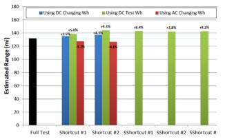
Figure 3: UDDS Cycle Range Extrapolation Results for Various Calculation Methods
