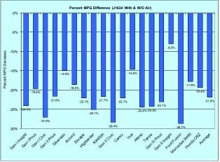
Figure 4. Percentage decrease in baseline performance fuel economy test results for SAE J1634 drive cycle testing when the air conditioning is turned on during the testing.
