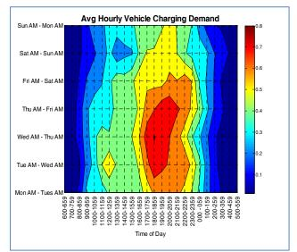
Figure 10. Average hourly charging demand for charging Hymotion Prius PHEV conversions for vehicles operated by households in California. Scale is from 0.1 to 0.8 (dark red) kW.
