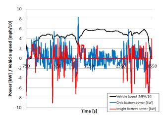
Figure 5. Usage of Hybrid System of an Insight Compared with a Civic Hybrid
