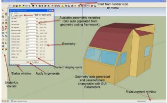
Figure 2. Parametric Cab Geometry Creation
