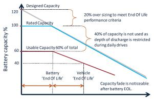
Number of discharge cycles Figure 4. Battery capacity variation with battery use
