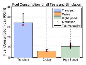
Figure 3. Simulation Results within Test-to-test Uncertainty
