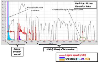
Figure 4. Hymotion Prius PHEV Emissions During Cold-Start UDDS Cycle
