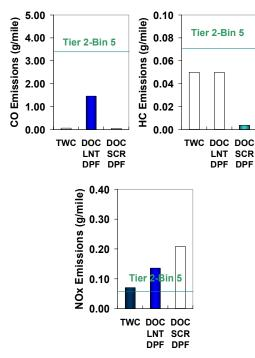
Figure 2. Comparison of cumulative tailpipe emissions from a conventional gasoline-powered passenger HEV with TWC and a diesel-powered HEV with different lean aftertreatment combinations. Simulations are for 80 consecutive UDDS cycles beginning with a cold start.
