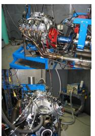
Figure 7. Dynamometer testing configuration for the circle track-525 LS3 engine (top and bottom). MAST Motorsports engine is shown on the right with the SEMTECH DS portable emissions measurement system (PEMS).
