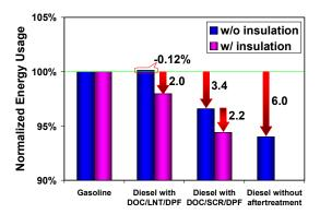
Figure 4. Impact of thermal insulation on the normalized energy usage of a gasoline passenger HEV with TWC and a diesel HEV with the different lean aftertreatment combinations. Simulations are for 80 consecutive UDDS cycles beginning with a cold start.
