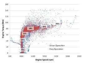
Figure 16. Urban and Highway Engine Usage and Efficiency
