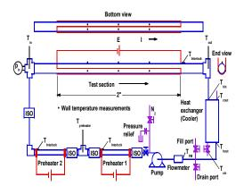
Figure 1. Test Facility Schematic Diagram
