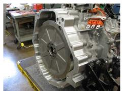
Figure 9. Torque Sensor Spacer
