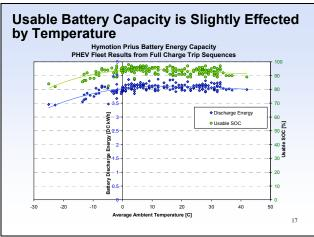
Figure 8. Usable battery capacity by temperature.
