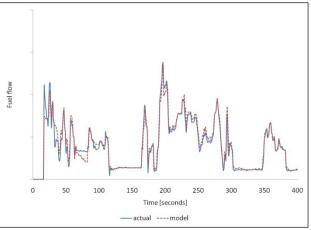
Figure 5. Cold-start model vs. actual fueling detail, initial oil temperature =  $20^{\circ}$ C, UDDS cycle. Tooolant = model input for engine temperature.
