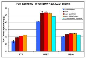
Figure 2. Fuel Economy and its Spread as a Function of Vehicle Mode and Drive Cycle.
