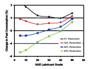
Figure 2: Predicted change in fuel economy as a function of engine lubricant viscosity and boundary friction for an off-road driving schedule (70% idle, mode 2 and 3).
