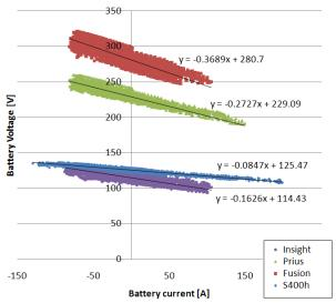
Figure 12: Different Battery Polarization Curve Comparisons
