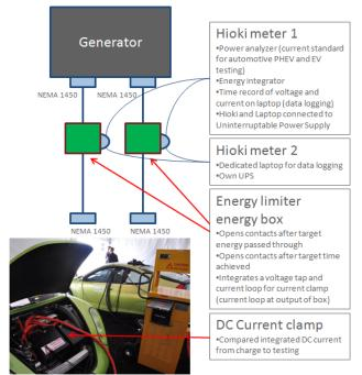
Figure 2. Charge set-up and instrumentation
