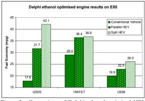
Figure 3. Comparison of Delphi ethanol-optimised HEV fuel economy results compared to Saab Bio-Power HEV
