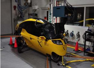
Figure 7. One of the two vehicles from Team X-tracer (#72 shown, #79 not shown) testing on the dynamometer
