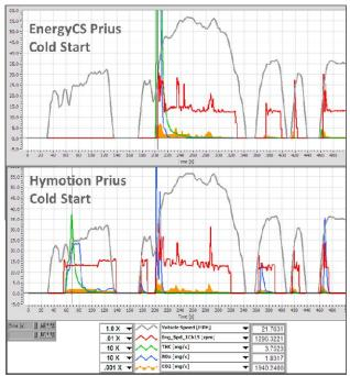
Figure 5.Comparison of Prius PHEV Initial Engine-Start Strategies in Cold-Start UDDS Cycle
