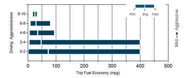
Aggressiveness factor is based on accelerator pedal position. The more time spent during a trip at higher accelerator pedal position, the higher the trip aggressiveness.
