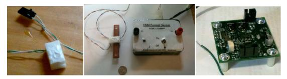
Figure 27 Flux-gate-magnetometer-based current sensor and signal conditioner
