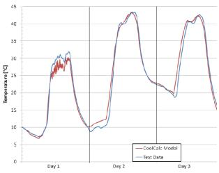
Figure 17. Cab Average Air Temperature Comparison
