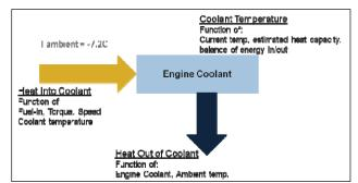
Figure 15. Preliminary coolant model overview.
