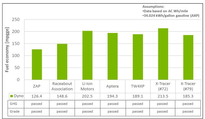
Figure 9. Dynamometer energy consumption results for the AXP validation stage
