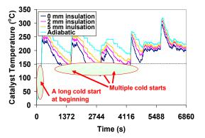
Figure 3. Impact of thermal insulation on urea-SCR catalyst temperature for a passenger PHEV under urban driving conditions.
