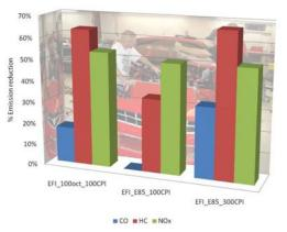
Figure 12. Catalytic convertor emissions reduction efficiencies, 100 CPI vs. 300 CPI (E85) vs. E85 (100 CPI) fuel-injected configurations.
