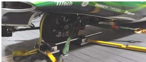
Figure 160. Three-wheel vehicle restraining system
