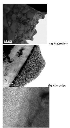
(c) Film-substrate interface Figure 2: a Tribochemical film from Lubricant A is amorphous.
