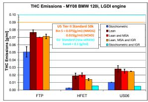
Figure 4. THC emissions as a Function of Vehicle Mode and Drive Cycle.
