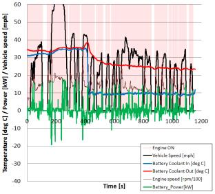
Figure 11: Forced Battery Pack Cooling Using the Airconditioning System
