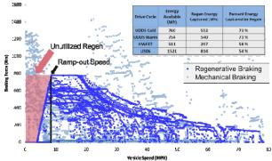
Figure 13. Estimated Regenerative Braking Envelope
