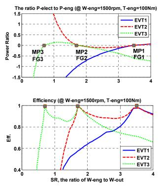
Figure 7. Power characteristics of the three-mode EVT with FGs
