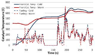
Figure 12. Cold versus Warm Front Catalyst Temperature and Fueling Rate
