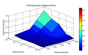
Figure 2. Total hydrocarbon engine out emissions on LAF engine
