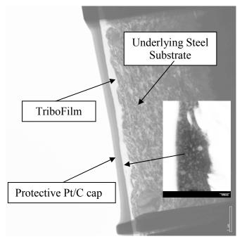
Figure 4. TEM image of tribofilm on steel block segment [4].
