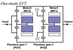
Figure 2. Schematic of the one-mode EVT
