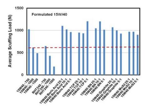
Figure 3: Average scuffing load of formulated 15W/40 and 15W/40 with additives.
