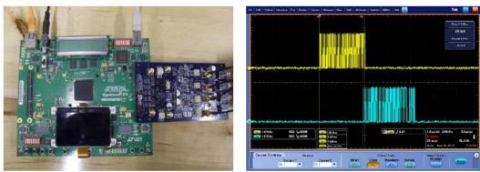
Altera Cyclone III FPGA development kit Modulate/demodulate bit stream Figure 25 Software-Defined Radio hardware and output waveforms
