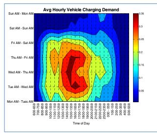
Figure 11. Average hourly charging demand for charging Hymotion Prius PHEV conversions for vehicles operated by commercial fleets in the United States. Note that the scale is different for the graphs for the commercial and private vehicles. The scale for this figure is from 0.05 to 0.35 (dark red) kW.
