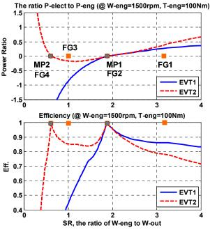
Figure 5. Power characteristics of the two-mode EVT with FGs  $% \left( {{F_{\mathrm{S}}} \right)^{-1}} \right)$
