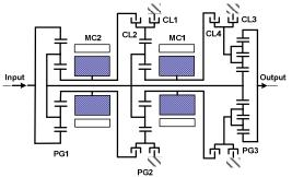
Figure 6. Schematic of the three-mode EVT with FGs
