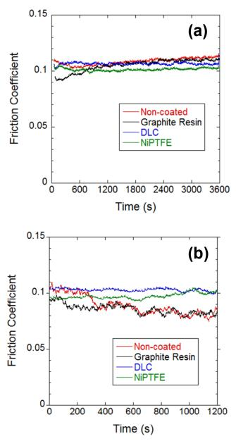
Figure 7: Friction coefficient as a function time for all samples tested using a load of 250 N in (a) fully formulated 10W30 oil at  $120^{\circ}$ C for 1 hour and (b) PAO10 oil at  $20^{\circ}$ C for 20 minutes.
