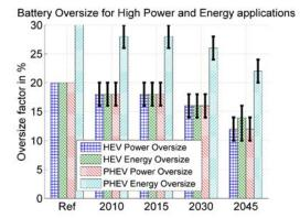
Figure 7. Battery Oversizing
