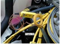
Figure 4. Engine Oil Temperature Sensor
