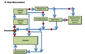
Figure 1. Main Cooling System Overview and Thermocouple Placement.
