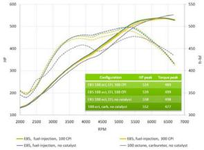
Figure 8. Engine dynamometer full-load, pull-testing results obtained at Mast Motorsports in November 2009.
