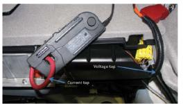
Figure 6. Position of Current Clamp and Voltage Tap
