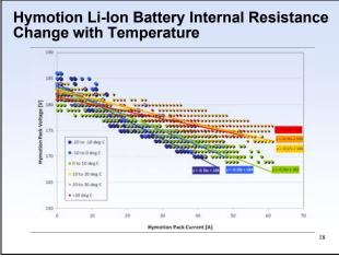
Figure 9. Hymotion Prius PHEV battery internal resistance change with temperature.
