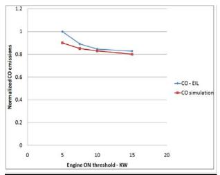
Figure 5: Comparison of CO trends for simulation and EIL.
