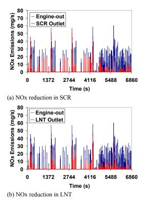
Figure 1. Comparison of tailpipe  $NO_x$  emissions between SCR and LNT catalysts for a diesel-powered passenger PHEV over five consecutive UDDS cycles beginning with a cold start.
