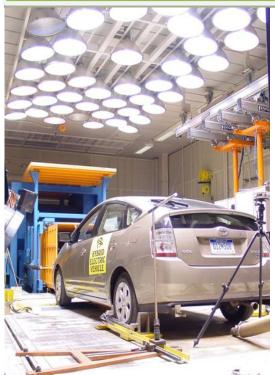
Figure 2. Photo of a test cell with solar spectrum
