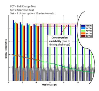
Figure 13: Full-charge Tests on the UDDS Cycle, Including the Short-cut Tests
