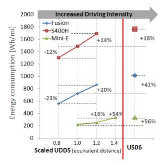
Figure 14: Drive Intensity Impact on Energy Consumption for Different Powertrains
