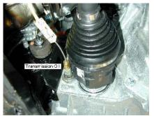
Figure 5. Transmission Oil Temperature Sensor
