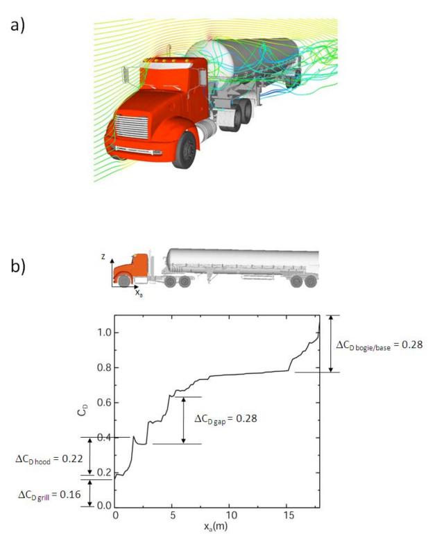
Figure 3. a) Velocity streamlines over a day-cab tractor and tanker trailer. b) Body-axis drag coefficient as a function of length along the tractor and tanker trailer.
