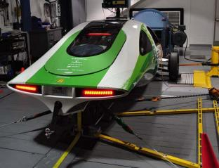
Figure 6. Team Aptera (#32) testing on the dynamometer
