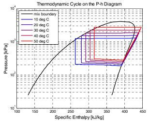
Figure 11. Output from A/C model shown on a P-h Diagram for a Series of Ambient Temperatures
