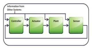
Figure 6: Generic component system configuration
