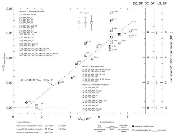
Figure 2. Reduction in the drag coefficient and estimated fuel usage for the various trailer skirts as a function of skirt area.
