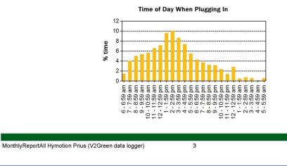
Figure 7. Page 3 of 3 for the PHEV summary report for 184 PHEVs operating April 2008 – September 2010 with onboard GridPoint data loggers.
