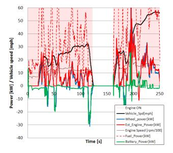
Figure 10: S400h Operation on a Hot-start UDDS
