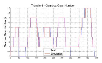
Figure 2: Gear Number Comparison on the Transient Cycle
