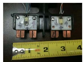
Figure 6. Flux-gate-magnetometer current sensor installed in low-cost UL-approved 60A-rated package
