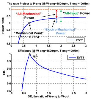
Figure 3. Power characteristics of the one-mode EVT
