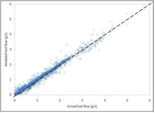
Figure 4. RSM BSFC model, predicted vs. actual data. R-squared values for the model = 0.98.
