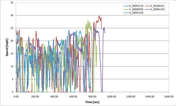
Figure 3. Transit Bus Highway Duty Cycles
