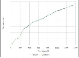
Figure 6. Model-predicted fuel consumed, 266 K UDDS cycle vs. actual recorded fuel consumed. Model < 0.4% predicted integrated value from actual data.
