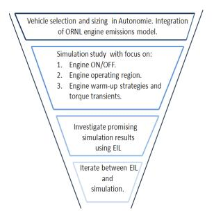
Figure 1. Model based design process
