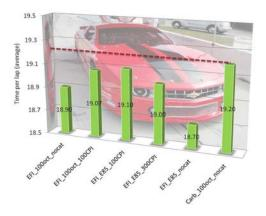
Figure 11. Results obtained on the New Smyrna 1/2-mile oval raceway. Bars indicate the average time per lap, in seconds, for each configuration.
