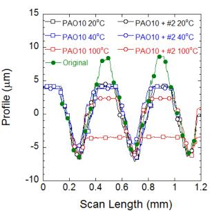
Figure 6: Wear measurements of samples tested using PAO10 and PAO10 containing 3 wt% BN/surfactant at 20°C, 40°C, and 100°C.
