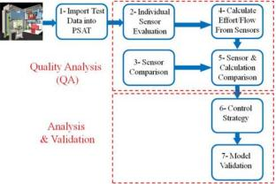
Figure 1. Test Data Analysis Process
