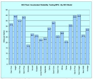
Figure 2. HEV fuel economy (mpg) test results for each HEV model in fleet and accelerated testing.
