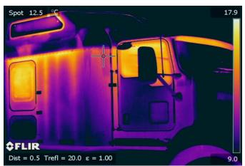
Figure 14. Infrared Image – Surface Temperatures
