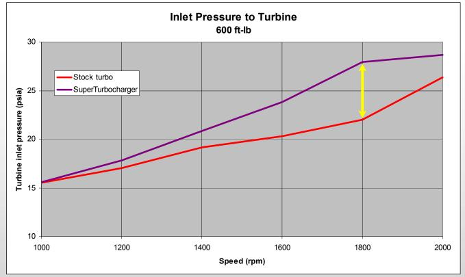
Inlet pressure to the turbine at 1800 rpm represents more pumping work lost with SuperTurbo
