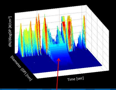
Particle distribution shifting to larger particle size
