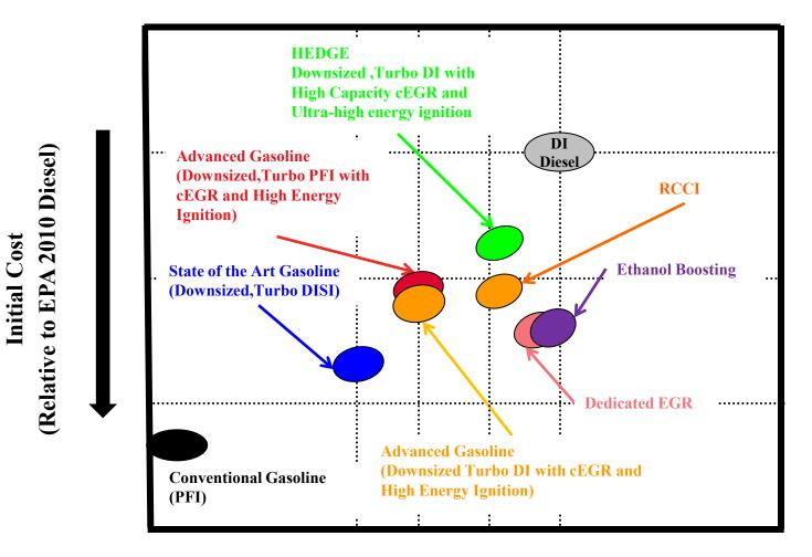
Increasing Brake Thermal Efficiency (Relative to EPA 2010 Diesel)
