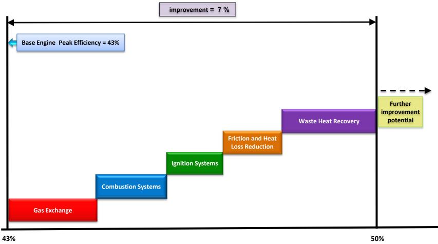
**Brake Thermal Efficiency (%)**
