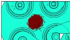
Flamelet kernals then generate the macroscopic flame kernel that initializes the combustion model
