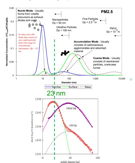
•D50=23 ensures soot particles are measured but limits detection of any nucleation mode particles that escape the evaporation tube.
