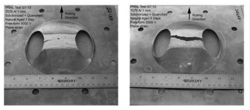
Figure III-24: Pictures of the pulse-pressure free-formed samples of AA7075 in W temper, 1-day (left) and 6-days (right) natural aged.
