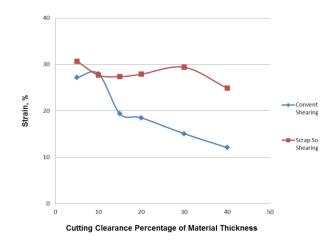
Figure III-32: Improved edge stretchability with scrap support.
