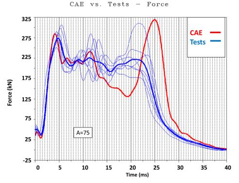
(a) Force-time history comparison of commercial code A to physical tests. Dark blue curve represents average of all physical tests.
