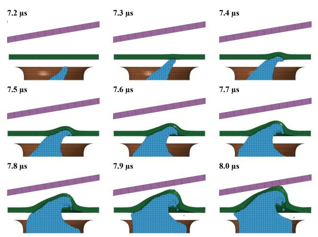
Figure III-82: Simulation of a 6.8kJ (13kV) EH pulse launching an AI 6022-T4 flyer into a DP600 steel target. A 70 µs offset is used on the time values.
