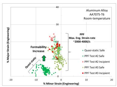
Figure III-26: FLD of AA7075-T6 under PPF and quasi-static bulge forming. Green symbols signify safe strains while red symbols signify unsafe strains.
