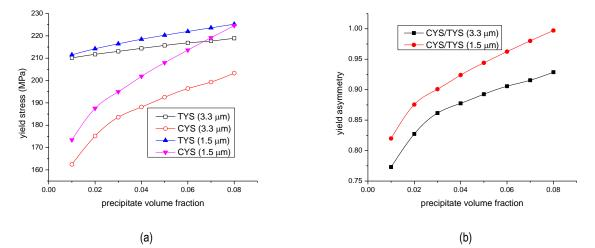
Figure III-35: Evolution of (a) yield strengths and (b) yield asymmetry with precipitate volume fraction when the precipitate size is kept constant.
