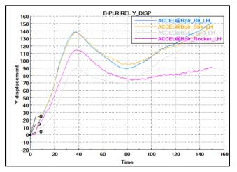
Figure V-7: MMLV FMVSS 214D Side Impact Results (units: x-axis msec, y-axis millimeters).
