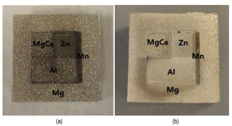
Figure III-133: Mg diffusion multiples for low temperature measurement. (a) 315°C for 790 hours; and (b) 275°C for 1760 hours.
