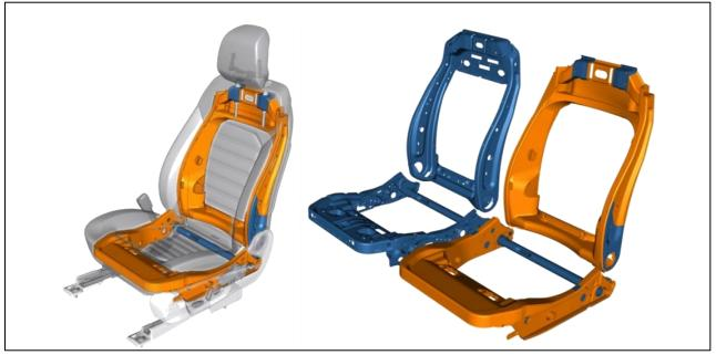
Figure V-15: CF Composite Seat Back and Cushion Structures (Production Steel Seat Structure Illustrated for Comparison).
