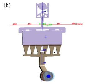
Figure III-150: Schematic illustration of die geometry for producing HPDC (a) AM60B and AZ91 at Tsinghua University and (b) AM70 at Ford Motor Co.
