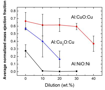
Figure V-49: The average normalized mass ejection as a function of dilution for different weight percents of Al:NiO, Al:CuO, and Al:Cu<sub>2</sub>O foils, where the diluent is the metal from the starting oxide.
