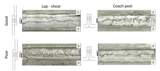
Figure III-5: Comparison of friction weld zone appearances for examples of good and poor welds in both lap-shear and coach peel geometries. AS= 'advancing side', RS='retreating side' of tool motion.
