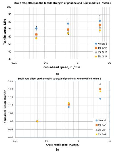
Figure V-57: Strain rate effect on pristine and GnP modified nylon-6: a) tensile strength, b) normalized tensile strength.
