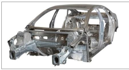
Figure V-3: Mach I BIW Prototype Build.
