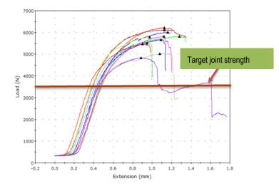
Figure III-56: Lap shear results of AZ31 Mg SPR joints created at elevated temperatures with an induction heat system.
