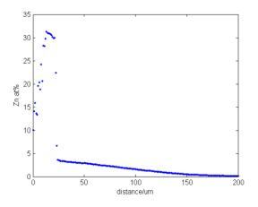
Figure III-129: Concentration profile measured using EPMA.
