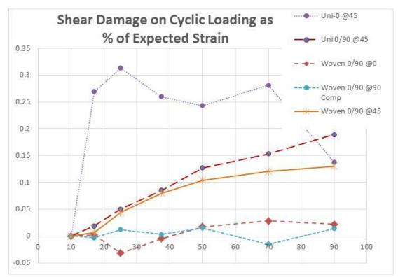
Figure IV-56: This chart shows the degradation of the shear properties of the unidirectional  $(0)_8$  and  $(0/90)_{28}$  and the woven  $(0/90)_{28}$  after cyclic loading at seven increasing strain loads. The unidirectional and woven materials tested at 45° degraded at an increasing pace, while the unidirectional  $(0)_8$  immediately lost considerable structure, and the woven tested in tension and compression show good resistance to the loading.
