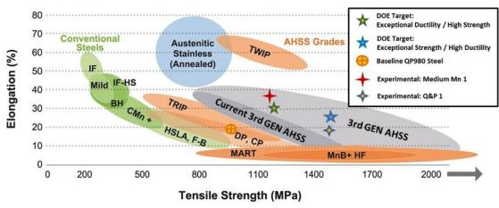
Figure III-9: 3GAHSS mechanical properties.
