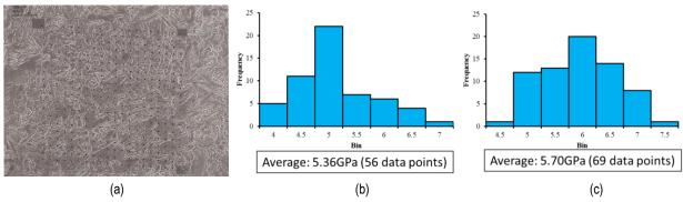
Figure III-22: (a) Nano-indentation test with MAT8, and some hardness results for tempered martensite in (b) MAT8 and (c) MAT10.
