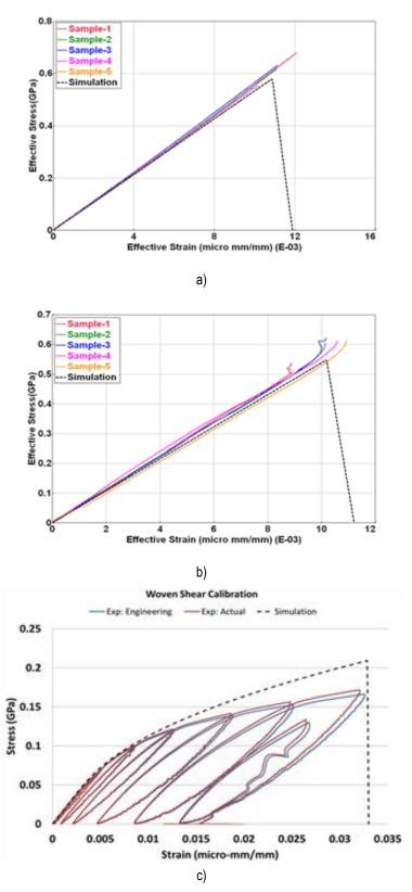
Figure IV-59: Material Model Calibration Results for PAM-CRASH Material 131 (a) Tension, (b) Compression, (c) Cyclic Shear.
