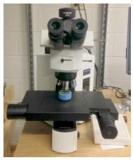
Figure IV-17: Optical microscope system with motorized stage for use in fiber measurements.
