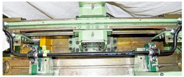
Figure V-25: Rear Stabilizer Bar Fatigue Test Setup.
