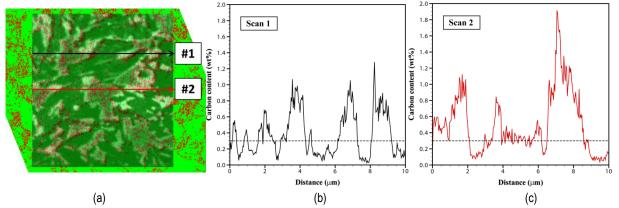
Figure III-19: (a) Overlay of carbon count image from nano-SIMS on EBSD phase map, (b) and (c) carbon distributons along the two lines.
