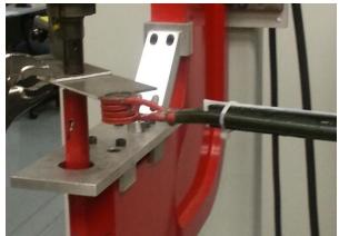
Figure III-55: Induction heating integrated into the Stanley Engineered Fastening SPR system for joining Mg sheet samples.
