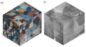
Figure III-110: Optical microstructure of Mg-2%Al alloy (a) and pure Mg (b) with three orthogonal directions. For Mg-2% Al alloy, the scale bar for every direction is the same and is 500  $\mu$ m. For pure Mg, the scale bar for every direction is the same and is 1000  $\mu$ m.
