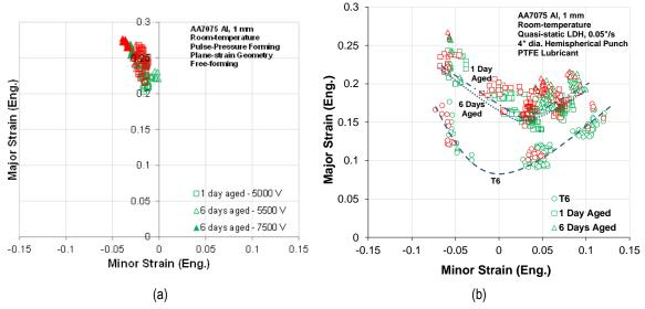
Figure III-25: (a) FLD of PPF AA7075 in W tempers. (b) Quasi-static FLC of AA7075 obtained by LDH tests. The dashed lines are meant to guide the eye and not indicative of any model or best fit. Green symbols signify safe strains while red symbols signify unsafe strains.
