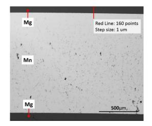
Figure III-123: Back-scattered Electron (BSE) image of the region labeled by red square in Figure III-122. The red line is for EPMA scanning.
