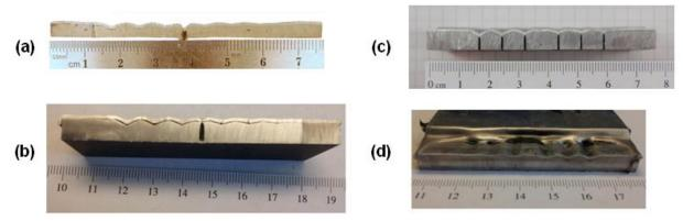
Figure V-76: Grooved target welds with material combinations and experimental conditions: (a) AA6061-T4/AM60B, no vacuum, (b) AA6061-T4/HSLA 656a, no vacuum, (c) AA6061-T4/HSLA 656a, slotted target, no vacuum, (d) AA6061-T4HSLA 656, AISI 1018 steel interlayer.
