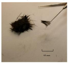
Figure IV-34: Selected PlastiComp sample showing longentangled fibers.
