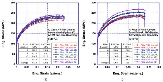
Figure III-43: Quasi-static stress-strain data of A-pillar covers in the (a) as-received and (b) paint-baked conditions. The specimens failed at an engineering (Eng.) strain somewhat greater than 23%. However, the failure strain exceeded the physical limits of the extensometer (extens.) and hence, extensometer strain >23% could not be recorded. As a result, the specimens "appear" to fail abruptly at 23% strain.
