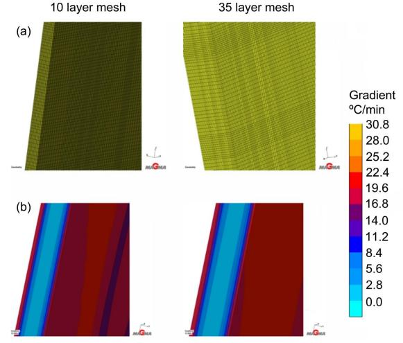
Figure III-151: MagmaSoft simulation of a plate casting with 2.5 mm thickness. (a) Refined meshes of 10 and 35 layers across the thickness; (b) Predicted local cooling rates using the refined meshes.
