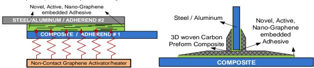
Figure V-52: LEFT: Schematic of the concept shown for in-plane joints, RIGHT: out-of-plane joints.
