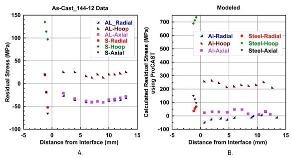
Figure III-79: A, measured, and B, predicted, residual stresses [MPa] for the as-cast condition.
