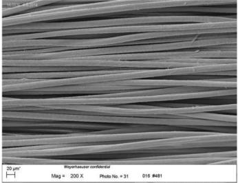
25% lignin/PAN precursor fiber from BP with standard co-monomer ratio – longitudinal view Figure IV-5: Precursor fiber sample #481.
