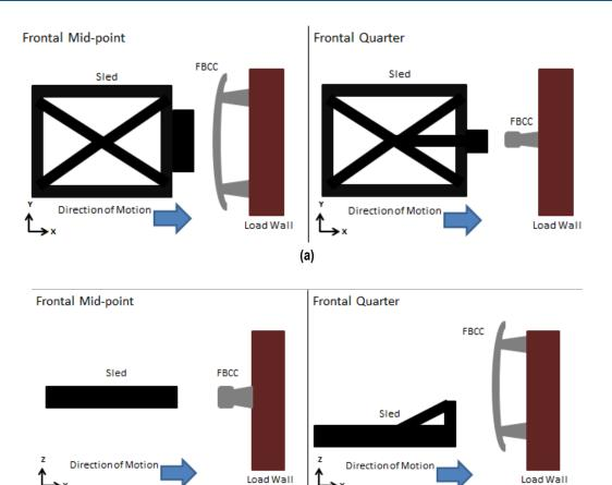
Figure IV-49: (a) Overhead schematic of low-speed tests; (b) Side schematic of low speed tests.
