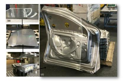
Figure III-62: Dissimilar thickness blanks produced at TWB for stamping trials showing production chain: (a) Welded blanks as produced, (b)welded blanks after laser cutting at Quality Measurement Control, Inc. (QMC Inc.), (c) laser-cut panels loaded for stamping at TWB, and (d) dissimilar thickness door inner panels after stamping showing 2-mm AA5083 welded to 1.1-mm AA5083.
