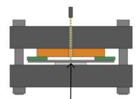
Vaporizing foil actuator (b)
