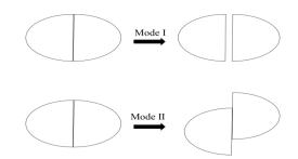
Figure III-36: Schematic illustration of the 2D version of Griffith's brittle failure criterion.
