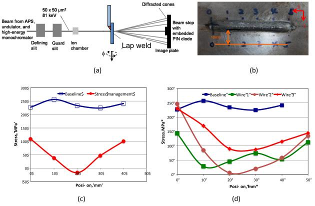
Figure III-76: High-energy synchrotron residual stress measurement. Transverse residual stresses are shown. (a) Synchrotron diffraction experimental setup. (b) Measurement locations relative to the stitch weld. (c) Reduction of weld residual stresses by means of proactive thermomechanical stress management. (d) Reduction of weld residual stresses by means of LTT weld wires with three different LTT wires and the baseline ER70-S weld wire.
