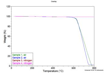
Figure IV-28: TGA of CFs with 5°C/min temperature increase in ambient air and in nitrogen.
