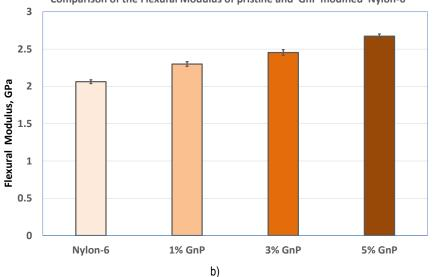
Comparison of the Flexural Modulus of pristine and GnP modified Nylon-6
