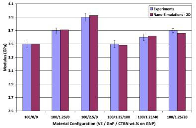
Figure V-64: Comparison of Experimental Modulus (E11) with Numerical Predictions.
