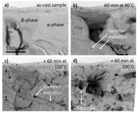
Figure III-146: TEM images of HPDC AZ91 alloy. a) As-cast sample showing the  $\alpha$ - and  $\beta$ -phase before heat treatment, b) after 60 minutes at 80°C, c) after an additional 60 minutes at 150°C, and d) after a further 60 minutes at 200°C. All figures are at the same magnification as indicated by the scale bar shown in (a).
