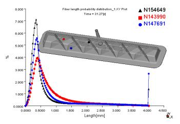
Figure IV-26: Example of 3D prediction of FLD for the complex part using five POD modes of the fiber breakage model based on unbreakable length: 150 segments,  $D_g = 3.0$ ,  $C_b = 0.02$ , S = 0.25.
