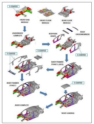
Figure V-4: Alternative Assembly and Corrosion Mitigation.
