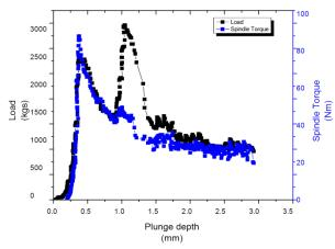
Figure III-39: Extrusion load and torque on the ram during the extrusion of ZK60 as a function of ram plunge depth.
