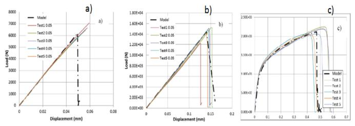
Figure IV-60: Material Model Calibration Results of the Microplane Model with Preferential orientations for (a) Tension, (b) Compression, (c) In-plane Shear ([0,90]<sub>2s</sub> laminate).
