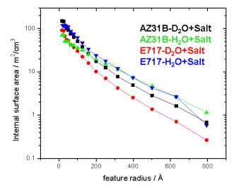
Figure III-68: Surface area distribution as a function of fitted feature radius size obtained from modeling the scattering data with a polydisperse hard sphere model (from reference 8).
