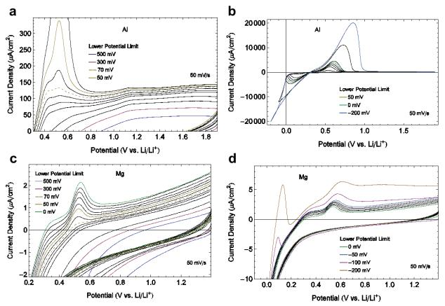
Figure III-92: Cyclic voltammetry performed at 50 millivolts per second (mV/s) in 1.0 molarity lithium perchlorate (M LiCIO<sub>4</sub>) in propylene carbonate at increasingly lower potential limits for a, b) Al sheet, 99.999%, and c, d) Mg, 99.95% sanded down to 1200 grit/p4000 in a UHP argon (Ar) atmosphere to minimize the native oxides. Significant traces are labeled by the CV lower potential limit (V) vs. Li/Li<sup>+</sup>.
