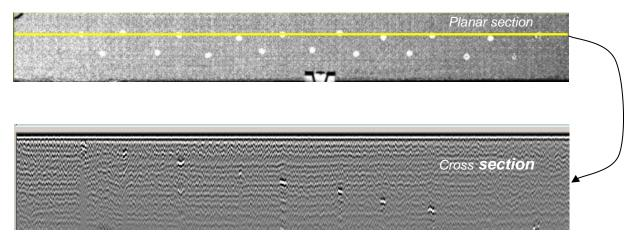
Figure IV-70: Ultrasonic images of an 11-ply woven carbon fiber composite with polyethylene (PE) and PTFE inserts. The upper image is the peak reflection within the material. The lower image is a cross-section showing the inter-ply locations of some of the PE inserts as well as some of the inter-ply and tow structure. Taken at 0.5-mm resolution using a pulsed 15-MHz transducer. Sample is 610-mm W x 75 H x 2.5 thick.
