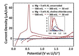
Figure III-101: Anodic stripping curves at 5 mV/s in 1.0 M LiCIO<sub>4</sub> in propylene carbonate following 600 second chronoamperometry at the lower potential limit: (dotted) 500 mV, (dashed) 300 mV and (solid) 50 mV vs. Li/Li<sup>+</sup> for  $\alpha$  Mg-5at% AI: (blue) un-corroded and (red) following potentiostatic corrosion at -100 mV vs. AI/AI<sup>3+</sup> for 60 min in a deep eutectic 1:2 molar ratio of choline chloride:urea at 150°C.
