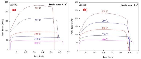
Figure V-43: Gleeble® test results for Mg AM60B alloy at high (>200°C) temperatures.
