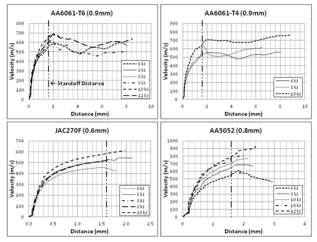
Figure V-74: Velocity vs Distance curves for each flyer material.
