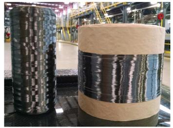
Figure IV-11: Typical spools of (a) 24 K industrial-grade carbon fiber and (b) 610 K rolls of textile-based carbon fiber.
