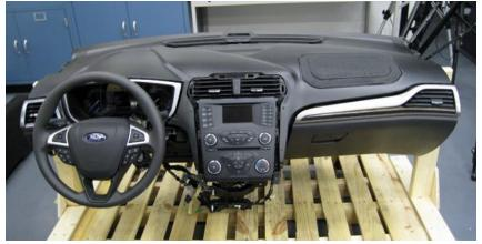
Figure V-21: Complete Carbon Composite MMLV IP/CCB.
