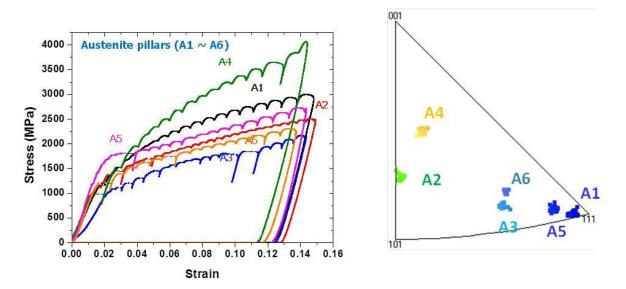
Figure III-12: Compressive micropillar stress-strain curves for the various single crystal orientations of austenite and the standard triangle showing the specific orientations for specimens A1-A6.
