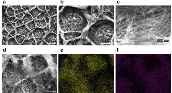
Figure III-100: Surface morphology using SEM of  $\alpha$  Mg-5at% AI following potentiostatic corrosion at -100 mV vs. AI/AI<sup>3+</sup> for 60 min in a deep eutectic 1:2 molar ratio of choline chloride:urea at 150°C shown at increasing magnification (a-c) as well as EDS areal mapping of the base, nanowire and ridge morphology shown in d) for e) Mg and f) AI abundance.
