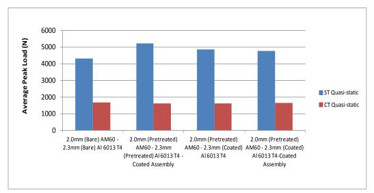
Figure V-37: Quasi-static shear tension and cross tension test results for selected coating configurations of Mg AM60B to Al6013 T-4 SPR joints.
