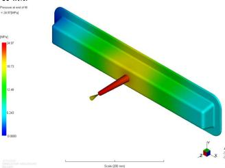
Figure IV-24: Distribution of pressure at the end of fill predicted for the 2.8 mm, 30-wt% LCF/PA66 complex part with ribs, including an acceptable level of the maximum pressure at the end of fill.
