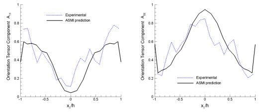
Figure IV-22: Predicted and measured fiber orientation tensor components in the flow- and cross-flow directions: (left) A<sub>11</sub>, (right) A<sub>22</sub>, for the edge-gated fast-fill 30-wt% LCF/PP plaque at location B.
