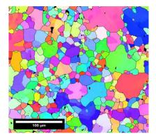
Figure III-49: An example of orientation imaging microscopy used to measure the grain size for each condition and location. This is the center of a HIP AM70 5mm plate. The black sections are Aluminum-Manganese (AIMn) intermetallics phases.
