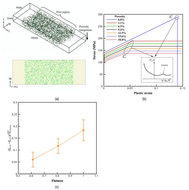
Figure III-52: (a) A 3D model with synthetic pore distribution (top) and the corresponding 2D model (bottom), (b) input properties for 3D and 2D model and (d) obtained 3D and 2D ductility correlation curve.
