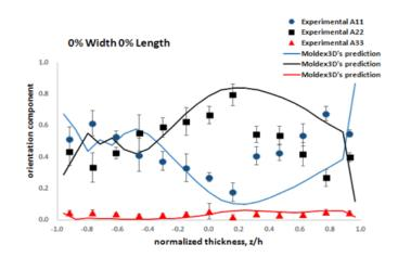
Figure IV-41: Measured points of fiber orientation taken at 10 locations on end-gated plaque.
