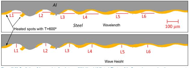
Figure III-85: Prediction of the wavy interface between 6061 AI and 1045 steel. The top of the figure shows wavelength measurements while the bottom shows wave height measurements. Yellow areas indicate localized regions where the temperature has exceeded the melting point of AI (600°C).
