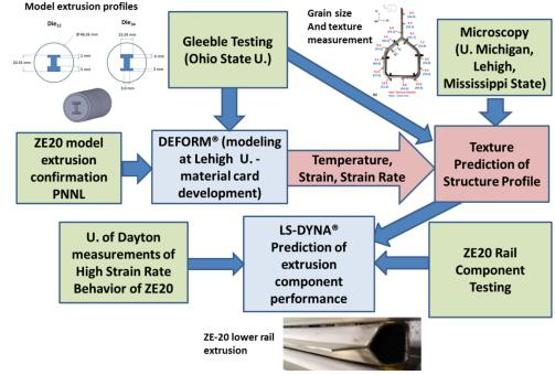
Figure III-8: Experimental and simulation information flows for the ZE20 extrusion modeling.
