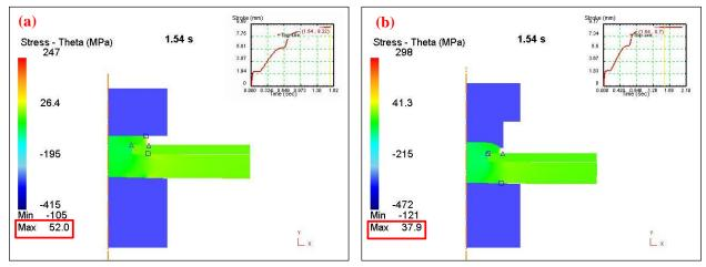
Figure V-44: Example simulation comparison of theta (hoop) stress created by two different electrode shapes.
