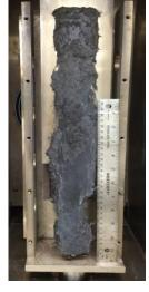
Figure IV-39: Sliding plate rheometer with a sample.
