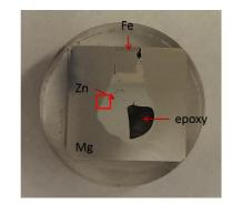
Figure III-126: The polished section of Mg-Zn diffusion multiple heated at 450°C for 8 hours.
