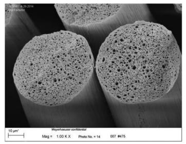
40% lignin/PAN precursor fiber from BP with standard co-monomer ratio – coagulated bath Figure IV-3: Precursor fiber sample #475.
