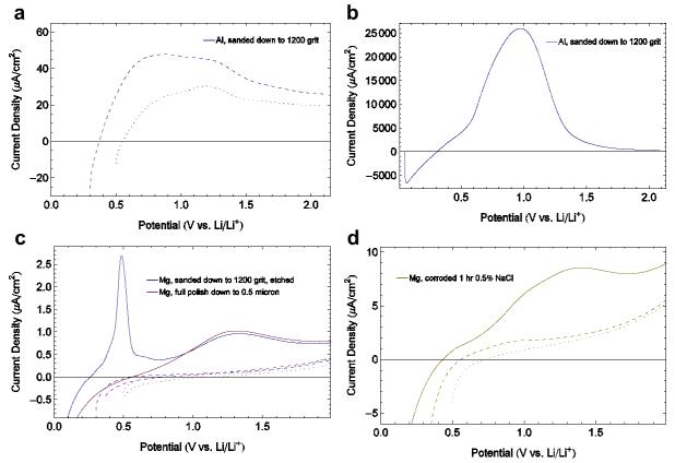
Figure III-93: Anodic stripping curves at 5 mV/s in 1.0 M LiCIO₄ in propylene carbonate following 600 second chronoamperometry at the lower potential limit: (dotted) 500 mV, (dashed) 300 mV and (solid) 50 mV vs. Li/Li<sup>+</sup> for a, b) AI sheet, 99.999%, and Mg, 99.95% for various preparations: c) sanded down to 1200 grit/p4000 vs. fully oil-based polishing down to 0.5 µm and d) corroded under full immersion in 0.5% aqueous NaCl for 1 hr.
