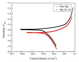
Figure III-111: Polarization curves for pure Mg and Mg-2% AI alloy in 3.5% NaCI solution.
