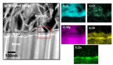
Figure III-69: Dark Field STEM of the film cross section (a) and corresponding energy dispersive spectrometry (EDS) elemental maps (b–f) generated from the boxed region for AZ31B after 4 h in H<sub>2</sub>O with 1 wt % NaCl (from reference 8).
