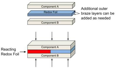
Figure V-45: A schematic representation of bonding with a Redox Foil. After ignition, the foil self-propagates through the bond interface.
