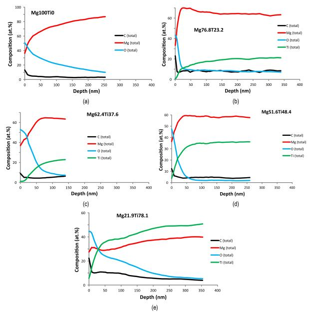
Figure III-114: XPS profiles for MgTi alloy surfaces in air.
