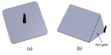
Figure IV-13: (a) Center-gated and (b) edge-gated 7 in x 7 in x 0.125 in PlastiComp plaque designs.
