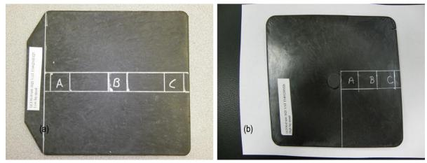
Figure IV-16: Locations A, B, and C defined on the (a) edge-gated and (b) center-gated plaques were isolated for shipping to Purdue for fiber orientation and length measurement.
