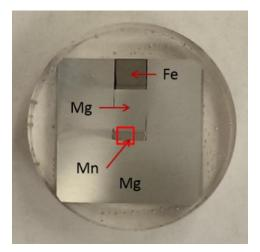
Figure III-122: The polished section of Mg-Mn diffusion multiple heated at 600°C for 48 hours.
