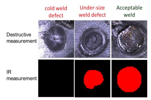
Figure III-73: Post-weld IR thermal signature vs. destructively measured weld nugget.
