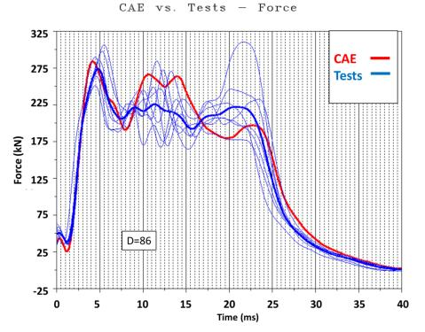
(d) Force-time history comparison of commercial code D to physical tests. Dark blue curve represents average of all physical tests.
