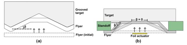
Figure V-72: Schematics of flyer collapse onto (a) grooved target, (b) flat target. It should be noted that the view in (a) is along the width direction of the foil actuator while (b) is a view along the length direction of the foil actuator.  $\beta$  is the dynamic collision angle.
