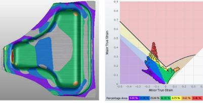
Figure III-13: Example showing T-Component formability simulation Linear Strain Path - 16mm draw home (courtesy of AK Steel).
