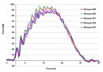
Figure IV-51: Impact force vs. time of frontal mid-point impact tests.
