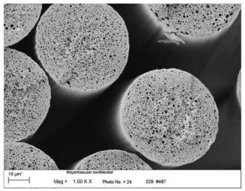
35% lignin/PAN precursor fiber from BP with standard co-monomer ratio – coagulated bath Figure IV-2: Precursor fiber sample #487.
