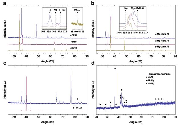
Figure III-91: XRD patterns for a) commercial alloys AZ91D, AM60 and AZ31B, b) solid-solution  $\alpha$  phase samples containing approximately 2-8 at% AI, c) Mg<sub>17</sub>AI<sub>12</sub>  $\beta$  phase with and without 1% Zn and d) MnAI<sub>3</sub>.
