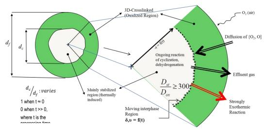
Figure IV-8: Single filament cross section during conventional oxidative stabilization process [4-6].
