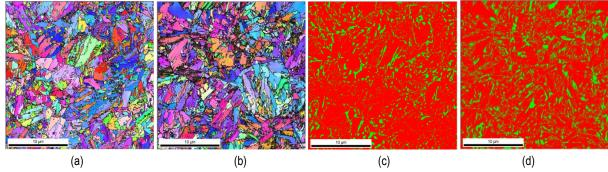
Figure III-20: Microstructure comparison between MAT8 and MAT9. Grain orientation maps of (a) MAT8 and (b) MAT9 and phase maps of (c) MAT8 and (d) MAT9.
