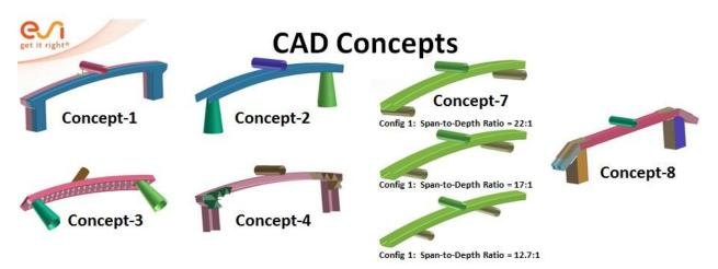
Figure IV-68: Composite Bumper Beam Concepts
