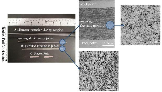
Figure V-46: Sequence of swaging and rolling steps. Typical microstructures of cross-sections taken from as-swaged and as-rolled AI:CuO samples are shown.
