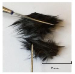
Figure IV-33: Selected ASPN fibers showing long-aligned fibers.
