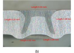
Figure III-57: Representative cross-section images of select 2 mm to 2 mm AZ31B SPR joints created at 300°C via the induction heat system. Interlock measurements are shown for a (a) flat-bottom die and (b) pip die.
