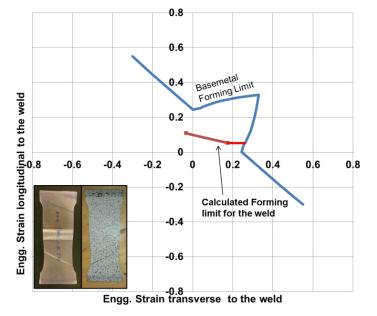
Figure III-63: Statistically calculated probabilistic formability limit diagram (red line) based on M-K method and experimental weld evaluation. Inset: A representative tensile sample showing typical failure in the thin sheet away from the weld line.
