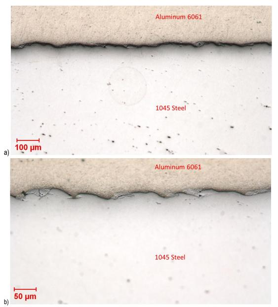
Figure III-86: Micrographs of an 18 kV (51.8 kJ) weld of an AI 6061-T6 extrusion welded to a 20° 1045CR steel mandrel. Images taken at (a) low and (b) medium magnifications.
