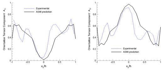
Figure IV-21: Predicted and measured fiber orientation tensor components in the flow- and cross-flow directions: (left) A<sub>11</sub>, (right) A<sub>22</sub>, for the edge-gated fast-fill 30-wt% LCF/PP plaque at location A.
