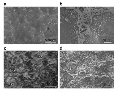
Figure III-102: Surface morphology using SEM of un-annealed Mg-8at% Al alloy: a,b) un-corroded and c,d) corroded at -100 mV vs. Al/Al<sup>3+</sup> for 30 min in a deep eutectic 1:2 molar ratio of choline chloride:urea at 150°C.
