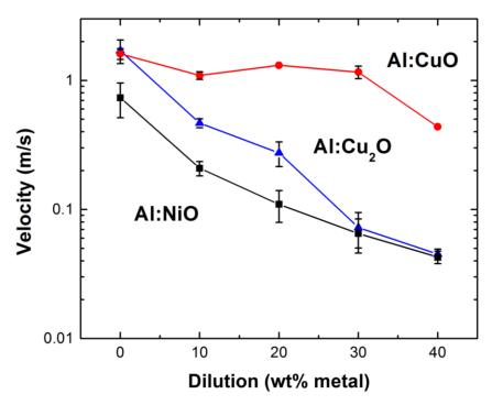
Figure V-50: Average propagation velocities of AI:NiO, AI:CuO, and AI:Cu2O foils as a function of dilution.
