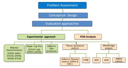
Figure V-54: Work-flow adopted to develop active adhesives.
