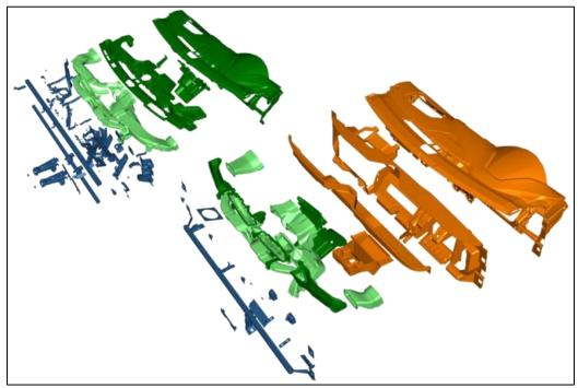
Figure V-18: CF IP/CCB Part Count Comparison.
