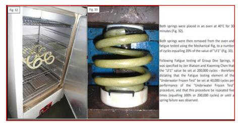
c) Springs Undergoing Heating Cycle and Fatigue Testing
