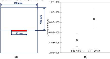
Figure III-74: Fatigue testing results with a new LTT wire compared with baseline ER70S-3 weld wire: (a) special weld fatigue specimen configuration and (b) fatigue testing results. R=0.1, f=10Hz.
