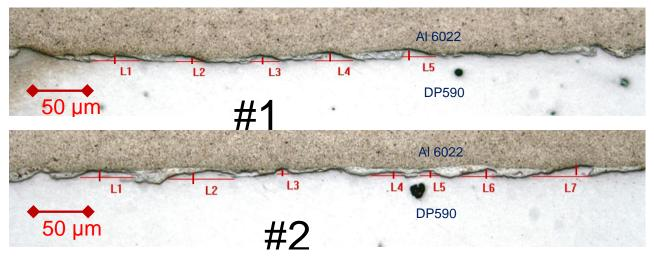
Figure III-87: EHP weld interface showing wavy interface of an EHP weld made at 6.8 kJ (13 kV) between 6022-T4 AI and DP600 steel at a 100 angle. Geometrical measurements of the wavy interface at the weld line were made at the marked locations for correlation with modelling.
