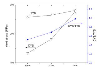
Figure III-33: Tension and compression yield stress and CYS/TYS along rolling direction for rolled AZ31 sheets with different grain sizes of 30  $\mu$ m, 10  $\mu$ m and 2  $\mu$ m, respectively[1].
