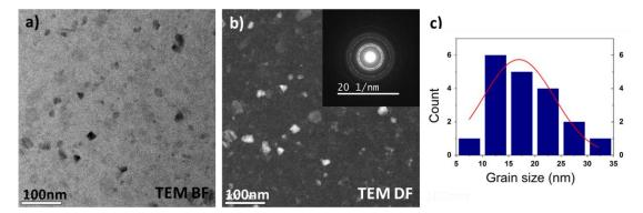
Figure III-144: a) TEM bright-field image of the Mg-9wt.% AI film. b) TEM dark-field image of the film, inset selected area diffraction pattern. c) Histogram showing the grain-size distribution in the film (blue bars) and a Gaussian fit to the histogram (red line) showing that the average grain size is between 15 and 20 nm.
