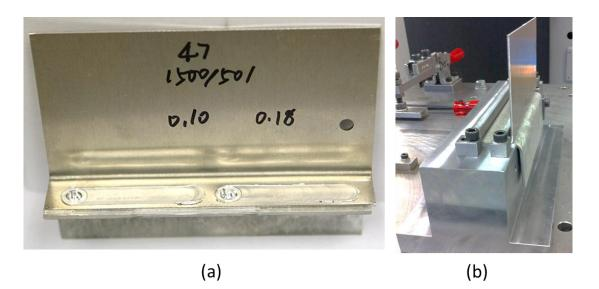
Figure III-3: (a) Example of the FSW "coach peel" joint between 6022-T4 AI and the AM60B Mg "top hat" casting wall portion and (b) fixture required to produce this joint.
