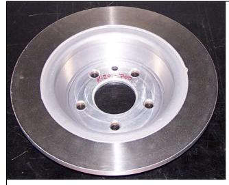
(a) Coated Rotor Prior to Test
