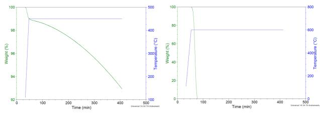
Figure IV-29: TGA analysis of CFs with a temperature increase held at 450°C in ambient air.
