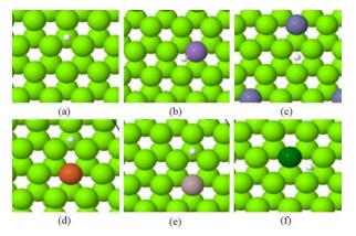
Figure III-105: Most favorable adsorption site of H on Mg-X(0001) with (a) X=Mg, (b) X=Mn, (c) X=Zn, (d) X=Fe, (e) X=AI and, (f) X=Ca.
