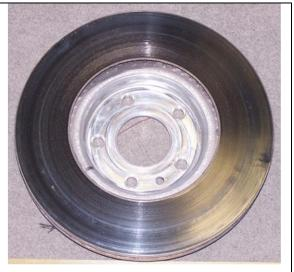
(b) Coated Rotor After Test
