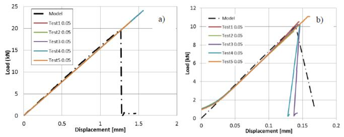
Figure IV-61: Material Model Calibration Results of the Microplane Model with Preferential orientations for (a) Tension, (b) Compression (Quasi-Isotropic configuration).
