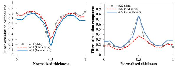
Figure IV-27: Comparison of fiber orientation data (from Wang 2007) with ASMI 3D predictions.
