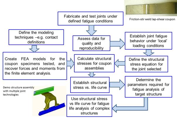
Figure III-4: Model development and data flow chart for development of the "structural stress" formalism for prediction of fatigue lifetimes for joint areas in complex structures such as the "demonstration".
