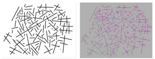
Figure IV-19: Automated identification and labeling of a sample image with multiple fiber crossings.
