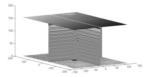
Figure IV-71: Ultrasonic images of an 11-ply woven carbon fiber composite subjected to impact with a standard hemispherical impactor. The top slice is the top indentation, while the other slices are the local reflectivity in three orthogonal planes and indicate the conical damage zone. Damage propagates from the bottom surface towards the front. There is no visible damage on the impacted top surface. The vertical height is exaggerated: the sample is 2.5 mm thick.
