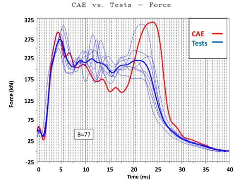
(b) Force-time history comparison of commercial code B to physical tests. Dark blue curve represents average of all physical tests.
