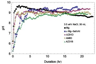
Figure III-98: Evolution of electrolyte pH of commercial alloys and common components under full-immersion, free-corrosion conditions in 3.5% aqueous NaCl using a standard glass electrode.
