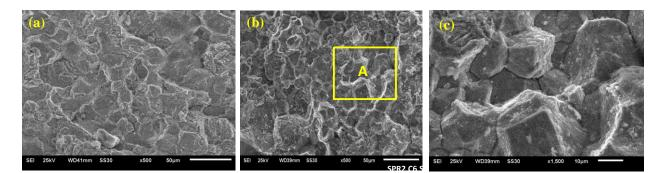
Figure V-41: SEM analysis of SPR joints failed after 6 weeks of ASTM G85-A2 accelerated corrosion exposure showing typical fracture morphology near inner surface of rivet.
