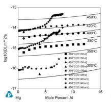
Figure III-135: Calculated interdiffusion coefficients in the Mg rich region of Mg-AI system along with the experimental data [6-8].
