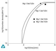
Figure III-136: Predicted number density of Mg<sub>2</sub>Sn precipitate in Mg-1.3 at.% Sn and Mg-1.9 at.% alloys along with the experimental data [9]
