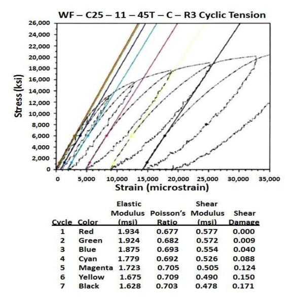
Figure IV-55: Cyclic tensile testing of carbon/epoxy twill weave  $(0/90)_{2s}$  plaques, tested at 45 degrees to partial strain in a cyclic manner. This test measures the shear damage induced in the sample by the cyclic loading.
