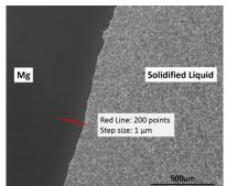
Figure III-127: BSE image of the region labeled by red square in Figure III-126. The red line is for EPMA scanning.
