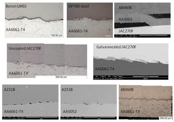
Figure V-77: Scanning electron and optical microscope images of the wavy welded interfaces between dissimilar materials (Note: UHSS is ultra-high strength steel).
