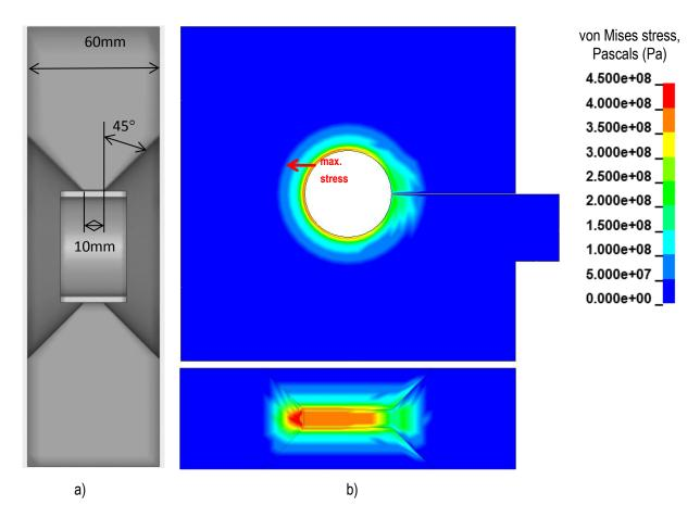
Figure III-80: Single-turn coil used for MPW of tubes: a) geometry, and b) von Mises stress levels during the discharge.
