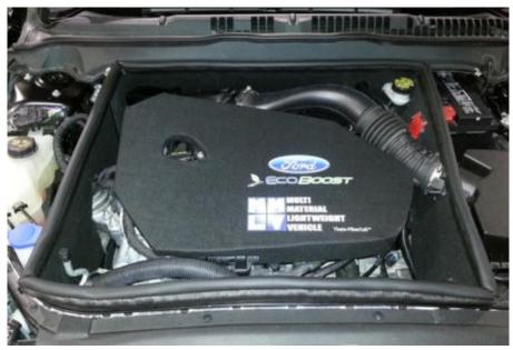
Figure V-26: Theta-Fiber™ Cell Engine Encapsulation and Engine Cover Prototype.
