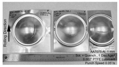
Figure III-23: Pictures of tested AA7075 specimens (solutionized + quenched +1 day natural aged) used to determine the corresponding forming limit curve (FLC) using the LDH tests.
