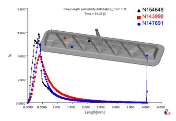
Figure IV-25: Example of 3D prediction of FLD for the complex part using the full fiber breakage model based on unbreakable length: 150 segments, drag coefficient,  $D_g = 3.0$ , shear rate constant,  $C_b = 0.02$ , and probability profile control factor, S = 0.25.
