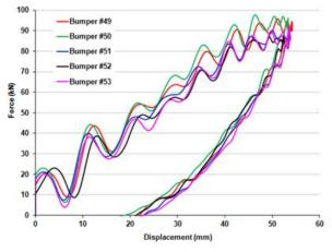
Figure IV-52: Impact force vs. displacement of frontal mid-point impact tests.
