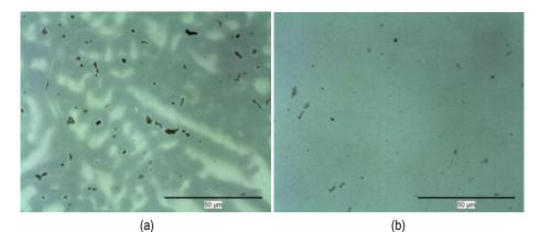
Figure III-142: Optical micrograph of Mg-2AI-8Sn alloy: (a) as cast; and (b) after solution treatment at 510°C for 70 hours. (Note the round Mg<sub>2</sub>Sn particles).
