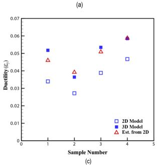
Figure III-53: Application of the developed 2D modeling methodolgy to actual pore distribution models. (a) An example of actual pore distribution (Song et al., 2009), (b) generated 3D model based on the actual pore distribution (top) and the corresponding 2D model (bottom) and (c) comparison of ductility estimated from 2D model and those of 3D model.
