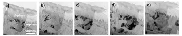
Figure III-147: TEM images of HPDC AZ91 alloy heat treated at 400°C. These images were captured in quick succession from a) to e) in less than 5 minutes, while the sample was heated to a maximum temperature of 400°C. The  $\beta$  phase is outlined in white in a). Scale bar for all images is as shown in (a).
