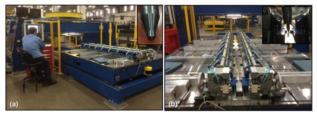
Figure III-61: High speed FSW equipment onsite at TWB Company, Monroe, MI. Machine and operator inside TWB plant with a typical tool used for welding is shown in the inset (a). Pneumatically controlled fixture for dissimilar thickness blanks. FSW tool attached to the machine head tilted to weld dissimilar thickness is shown in the inset (b).
