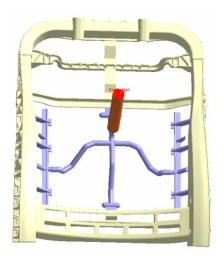
Figure IV-45: Model of complex part including the existing runner system.
