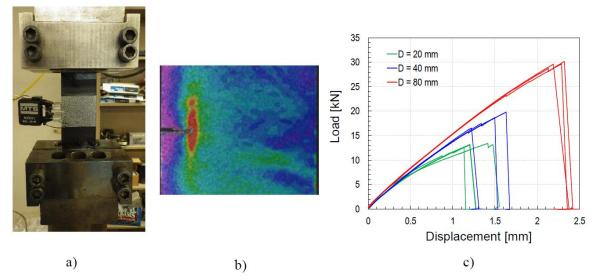
Figure IV-65: (a) Medium size SENT specimen under tensile loading in Crack Mouth Opening Displacement (CMOD) control, (b) Contour plot of the maximum principal strain measured by DIC used for model calibration, (c) Force-displacement curves for all the investigated sizes.
