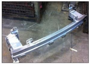
Figure V-10: MMLV Prototype Front Bumper.
