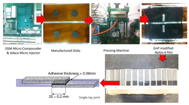
Figure V-56: Processing of 'pristine' and 'GnP-modified' nylon-6 films.
