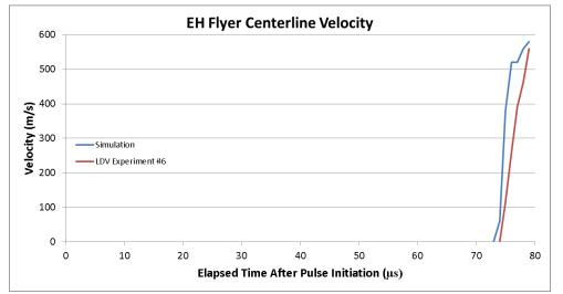
Figure III-83: Comparison of experimental and simulation derived velocities for an AI 6022-T4 flyer plate launched by a 6.8kJ (15kV) EH pulse.
