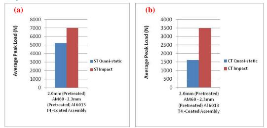
Figure V-38: Comparisons of quasi-static vs impact performance for shear tension (a) and cross tension (b) for pretreated Mg AM60B to Al6013 T-4 SPR joints.
