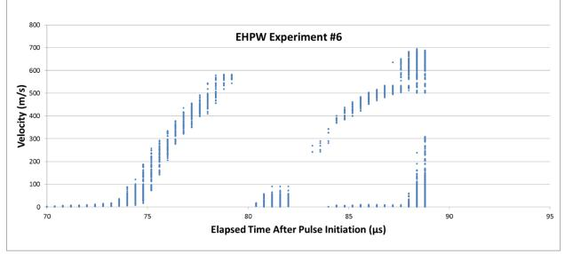
Figure III-88: Flyer plate velocity resulting from a 6.8 kJ (13 kV) EH discharge. The first peak is the flyer as it approaches the anvil, and the second peak is that of the Al plug. The flyer reached a velocity between 550-600 m/s before impact.
