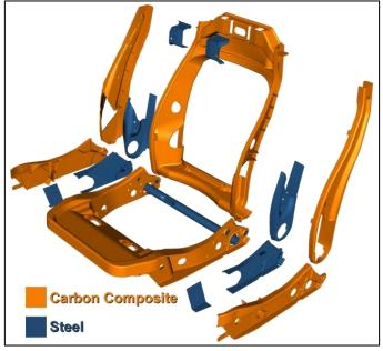
Figure V-16: CF Composite Seat Parts and Material Break Up.
