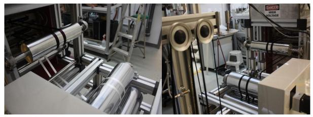
Figure IV-9: Processing two commodity-grade, 24,000-filament tows of precursor fiber in the large reactor.
