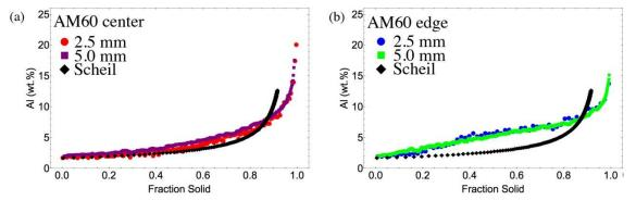
Figure III-156: Thickness effect on microsegregation behavior in AM60 at (a) center-line and (b) edge of plate.
