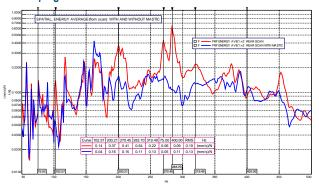
Figure V-30: Rear Floor Laser Scan Results Plot Of Spatial Energy Average Over All Scan Points. The Red Curve is Bare Floor Panel Before Damping Treatment and the Blue Curve is After Application of Damping Treatment.
