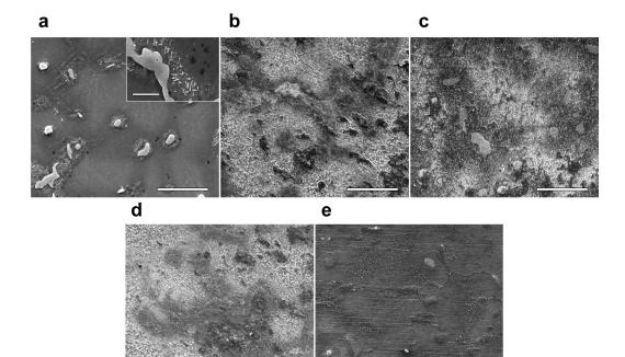
Figure III-96: Surface morphology using SEM of AZ91D: a) un-corroded, and corroded by full-immersion, free-corrosion in 3.5% aqueous NaCl for b) 5 min, c) 20 min, d) 4 hr and e) 20 hr. The inset of a) shows the Mg<sub>17</sub>Al<sub>12</sub>  $\beta$  phase surrounded by a eutectic region located at the grain boundaries. The scale bars are 50 µm for the main images and 10 µm for the inset.
