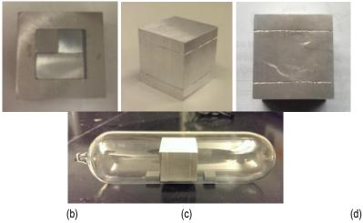
Figure III-121: The preparation procedure of solid diffusion multiples: (a) assembly; (b) welded; (c) hot- isostatically-pressed; and (d) encapsulated in a quartz tube.
