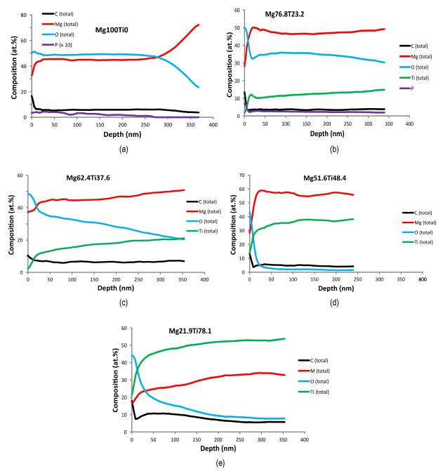
Figure III-115: XPS profiles for MgTi alloy surfaces after 24 h immersion in saturated Mg(OH)<sub>2</sub> + 0.1wt.% NaCl solution.
