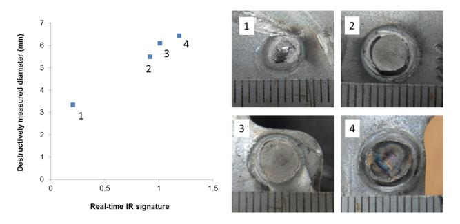
Figure III-72: Real-time IR thermal signature vs. destructively measured weld nugget size from an actual body component.
