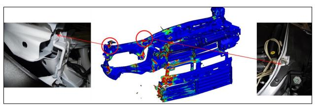
Figure V-32: CAE-vs.-Test Comparison in LSD – Example of Grill Opening Reinforcement Module Damage.
