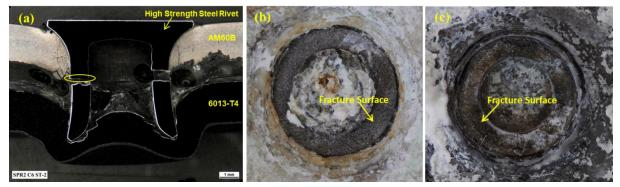
Figure V-40: SPR joint failure after 6 weeks of ASTM G85-A2 accelerated corrosion exposure.
