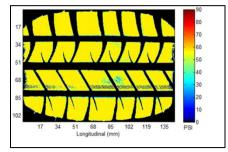
Figure V-22: Contact Patch of MMLV Tire.
