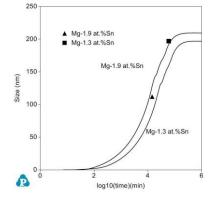
Figure III-137: Predicted radius of Mg<sub>2</sub>Sn precipitate in Mg-1.3 at.% Sn and Mg-1.9 at.% alloys along with the experimental data [9].
