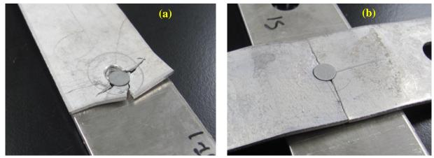
Figure V-36: Preliminary test samples of SPR Mg AM60B to Al6013 T-4 joints.
