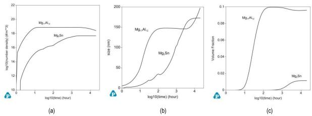
Figure III-141: Predicted (a) number density; (b) size; and (c) volume fraction of Mg<sub>17</sub>Al<sub>12</sub> and Mg<sub>2</sub>Sn precipitates in Mg-7Al-2Sn alloy at 200°C.
