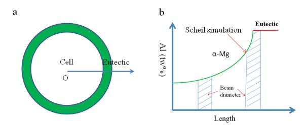
Figure III-154: Illustration of Monte Carlo simulation of the EPMA characterization of microsegregation: a) model of HPDC as-cast microstructure, b) illustration of the one-dimensional distribution of Al across a Mg cell from the center of the cell to the eutectic region.
