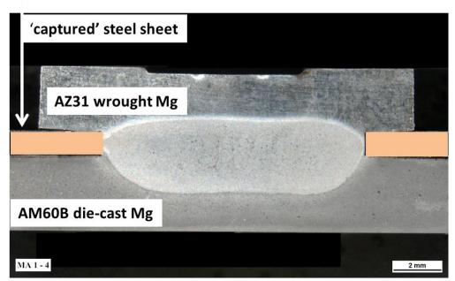
Figure III-2: Cross-sectional image of adaptable insert resistance weld joint between Mg and galvanized steel (colorized to highlight the location of the captured steel sheet member).
