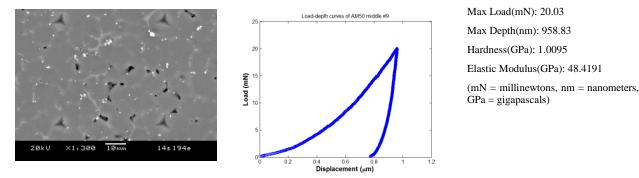
Figure III-51: Sample SEM image, loading-unloading curve, and machine output from nano-indentation experiment on AM50 as-cast sample.
