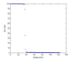
Figure III-124: Concentration profile measured by EPMA.
