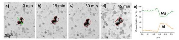
Figure III-148: TEM images of a  $\beta$ -phase particle (outlined in red) in Mg-9 wt.% Al film heat-treated at 400°C after a) 0 minutes, b) 15 minutes, c) 30 minutes, and d) 45 minutes. e) Electron energy loss spectroscopy (EELS) line profile across the original particle along the green arrow in a).
