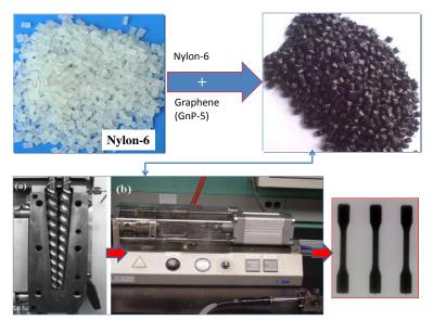
Figure V-55: Manufacturing process of pristine and GnP-modified nylon-6 coupons.
