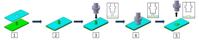
Figure V-33: Initial conceptual schematic of UPJ process – assembling parts, applying heat and force, assembly complete.
