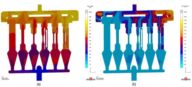
Figure III-46: MAGMASOFT® simulation results showing differences in (a) Flow Length and (b) Air Entrapment
