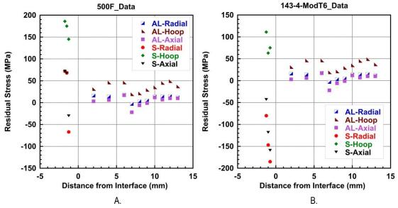
Figure III-78: The residual stresses as a function of distance from the interface for the 500°F (A) and modified T6 samples (B).
