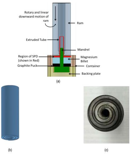
Figure III-38: (a) Diagram of the SAIE process and (b,c) shows the scrolls on the face of the ram which assists in heating and flow of material.
