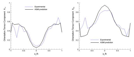
Figure IV-23: Predicted and measured fiber orientation tensor components in the flow- and cross-flow directions: (left) A<sub>11</sub>, (right) A<sub>22</sub>, for the edge-gated fast-fill 30-wt% LCF/PP plaque at location C.
