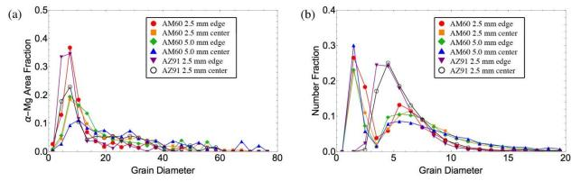
Figure III-153: Grain size distribution in the HPDC AM60 and AZ91 plates, represented as (a) the fraction of indexed area filled by grains of a given diameter and (b) the number fraction of grains with a diameter less than 20 µm.
