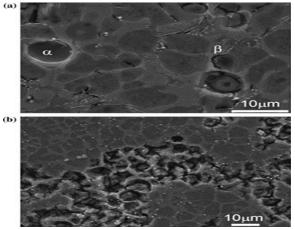
Figure III-108: Scanning electron micrographs of polished AE44 coupons at different times during the immersion test. Corrosion of the polished AE44 surface at two different times. Notice two types of corrosion present: (a) pitting and (b) intergranular corrosion [5].
