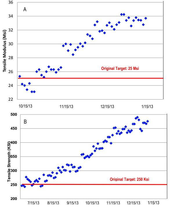
Figure IV-10: Progression over time of tensile modulus and tensile strength of carbon fiber produced from the Kaltex precursor during the project; (A) modulus progression and (B) strength progression.
