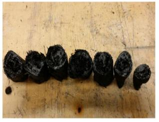
Figure IV-32: Nonuniform profile and voids within ASPN purges.
