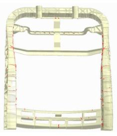
Figure IV-47: Visualization of weld lines in the front section of the complex part.
