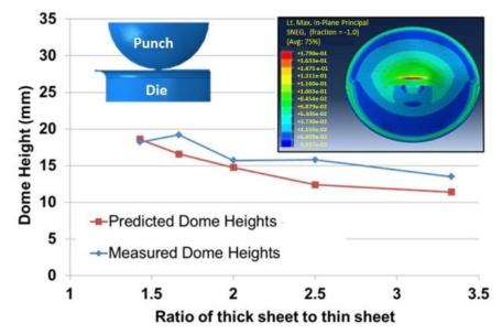
Figure III-64: Experimentally measured dome height and predicted dome height from computational model for various sheet thickness ratios. Inset: A representative strain map obtained from model showing strain localization outside of the weld line.
