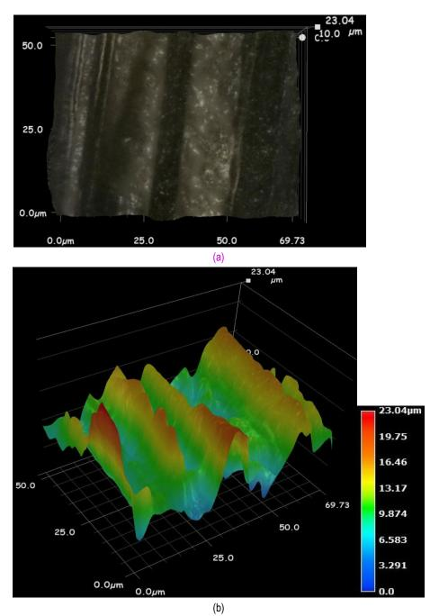
Figure V-70: Surface analysis for a laser-ablated Plasan CFPC specimen: (a) micrographs and (b) 3D scanning depth profile showing that the ablated thickness is 23 µm.
