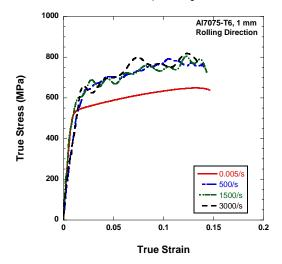
Figure III-27: Room-temperature uniaxial tensile stress-strain data for AA7075-T6 at quasi-static and high-strain-rates.
