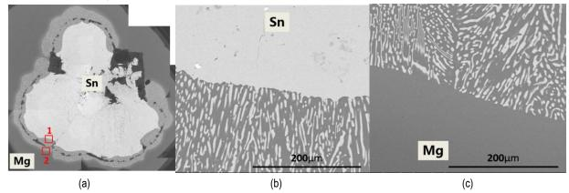
Figure III-132: BSE image of the Mg-Sn diffusion multiple heat treated at 550°C for 8 hours. (a) the whole region; (b) local region labeled by red square 1; and (c) local region labeled by red square 2.
