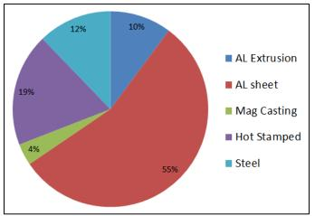
Figure V-8: MMLV Mach I Door Materials 65% AI, 21% Steel and 4% Mg.
