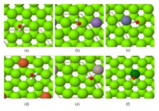
Figure III-104: Most favorable adsorption site of  $H_2O$  on Mg-X(0001) with (a) X=Mg, (b) X=Mn, (c) X=Zn, (d) X=Fe, (e) X=AI and, (f) X=Ca.
