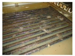
Figure IV-1: Heater coil in pre-stretching bath saturated with non-soluble residue during commercial spinning trial
