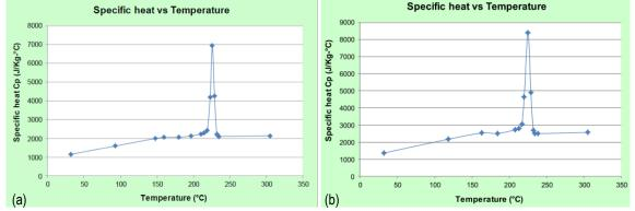
Figure IV-15: Specific heat vs. temperature curves recorded during cooling for (a) 30-wt% LCF/PA66 and (b) 50-wt% LCF/PA66 materials.
