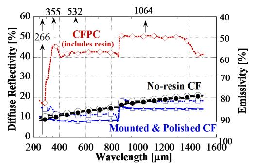
Figure V-65: Diffuse reflectivity data for the CFPC samples considered showing variations in the percentages of diffuse reflectivity and emissivity for over several wavelengths in microns (µm).
