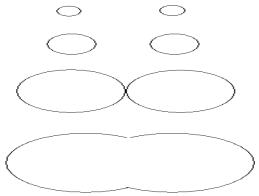
Figure III-109: Impingement coalescence illustrated by Horstemeyer [6].
