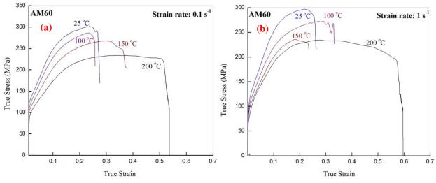
Figure V-42: Gleeble® test results for Mg AM60B alloy at low (<=200°C) temperatures.
