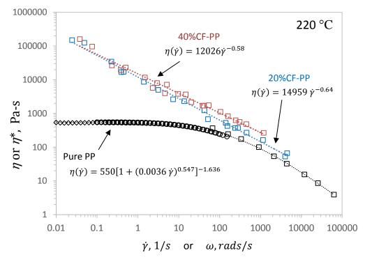
Figure IV-40: Viscosity versus shear rate data for the pure matrix (black) and 20 wt % (blue) and 40 wt % (orange) CF suspensions in PP. Data were obtained by cone and plate steady shear ( $\diamond$ ), cone and plate small amplitude oscillatory ( $\circ$ ), and capillary ( $\Box$ ) measurements.
