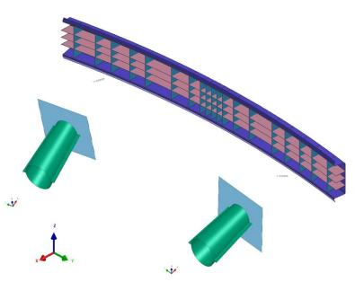
Figure IV-58: Tentative designs for the crush cans made from two compression-molded conical hat sections joined at the flanges, and the bumper beam, a C-channel with ribs on the included side, also compression molded.
