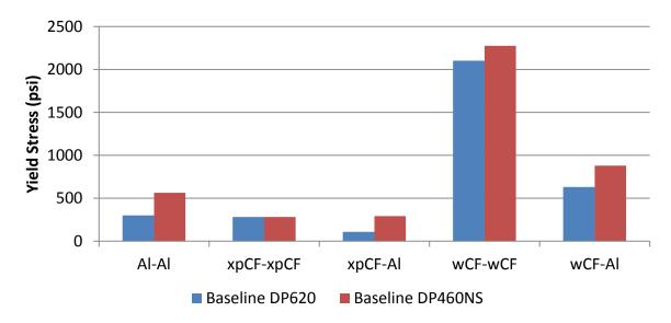
Figure V-66: Baseline single-lap shear results for DP620 and DP460 adhesives. (xpCF—cross-ply carbon fiber composite; wCF— woven carbon fiber composite).
