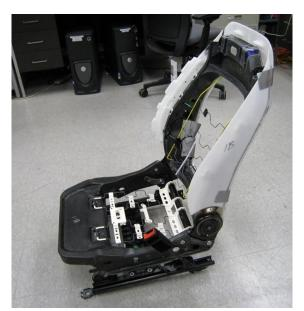
Figure V-20: CF Composite Prototype Seat.
