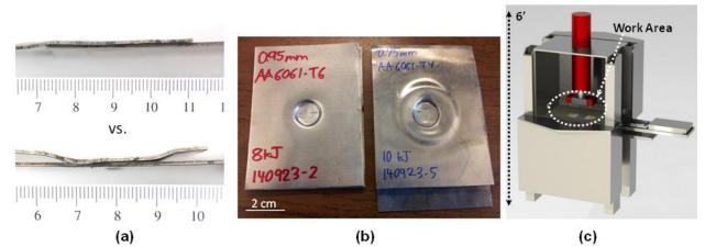
Figure V-79: Efforts toward technology transfer: (a) lap weld without overhangs, (b) spot weld, (c) a schematic of the automated VFAW system.
