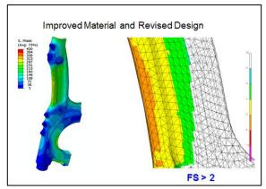
Figure V-13: Bulkhead Insert Fatigue Analysis.
