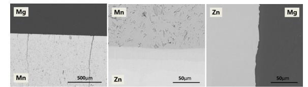
Figure III-134: BSE images of three diffusion systems in the diffusion multiple heated at 315°C for 790 hours.
