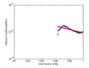
Figure III-130: Comparison of the interdiffusion coefficients obtained from the forward simulation [1] (red lines) with those obtained by the Sauer-Freise method [5] (blue lines).
