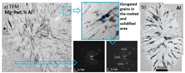
Figure III-145: a) TEM image of the laser-shot region in Mg-9wt.% Al film showing the elongated grains in the melted and solidified area and the diffraction patterns of the as-deposited structure and (0001) pattern of one of the grains in the as-cast microstructure. The circle in the cut-out shows the region imaged by the selected area aperture. b) Laser-melt/solidified pool in an Al film taken from Kulovits et al [5].
