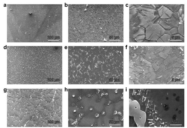
Figure III-89: Microstructural characterization of commercial alloys at various magnifications using SEM for a, b, c) AZ31B, d, e, f) AM60 and g, h, i) AZ91D. The alloys were prepared using oil-based polishing materials down to 0.5 µm and etched using acetic picral solution to expose grain boundaries and phases.
