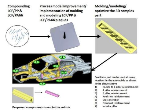
Figure IV-12: Schematic picture illustrating the technical approach to integrate and validate the tools for designing injection-molded LCF thermoplastic automotive structures.
