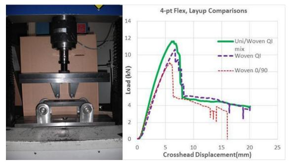
Figure IV-57: Configuration of the 4-pt flex test and comparison of the three layups. Curves are an average of 4 parts per layup. The sawtooth effect at the end of the displacement is an artifact of the averaging.
