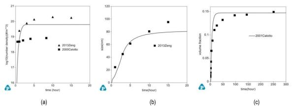
Figure III-140: Predicted (a) number density; (b) size; and (c) volume fraction of Mg17Al12 precipitate in Mg-9Al-1Zn alloy at 200°C with the experimental data [10-12].
