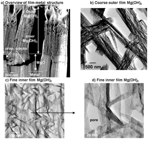
Figure III-67: AZ31B after 24 h in D<sub>2</sub>O with 5 wt % NaCI: a) assemblage of multiple HAADF STEM images of film-metal structure; bright field (BF) STEM images of coarse outer (b) and finer inner (c, d) Mg(OH)<sub>2</sub> (from reference 8). Cracks in structure are attributed to sample preparation.
