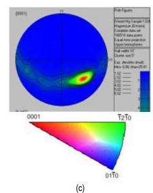
Figure III-41: (a) Optical image showing the ZK60 tube longitudinal cross-section at the central region of formed tube and (b) Inverse pole figure (IPF) of the same region and (c) texture analysis of the same.
