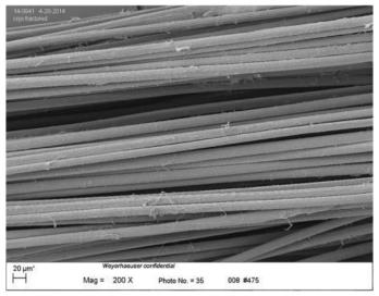
40% lignin/PAN precursor fiber from BP with standard co-monomer ratio - longitudinal view
