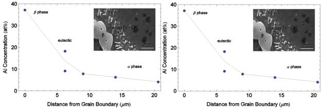
Figure III-90: Distribution of AI concentration in a balance of Mg within a representative AZ91D grain. The Mg<sub>17</sub>AI<sub>12</sub>  $\beta$  phase is proximal to the grain boundary, a solid solution  $\alpha$  phase 4-8 at% AI is located inside the grain, and between the two phases, a eutectic region exists consisting of both  $\alpha$  and  $\beta$  phases. The lowest AI concentration is found at the center of the grain, and it gradually increases outward toward the grain boundaries.
