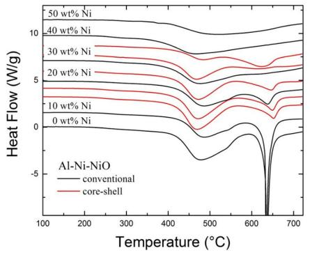
Figure V-47: DSC traces of loose compacts of AI, NiO, and Ni powders for various Ni dilutions. Exothermic reactions are identified by a negative heat flow. However, most curves are offset vertically for clarity.
