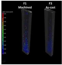
Figure III-47: CT scans of flat tensile bars indicating differences between porosity levels in machined and as-cast samples.
