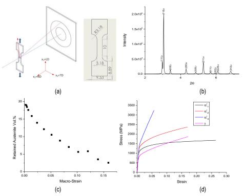
Figure III-17: (a) Schematic of experimental setup for in-situ HEXRD tests under uniaxial tension, (b) intensity vs. 20 profile integrated from diffraction rings, (c) austenite volume fraction evolution and (d) phase stress-strain curves estimated from EPSC model for MAT1.
