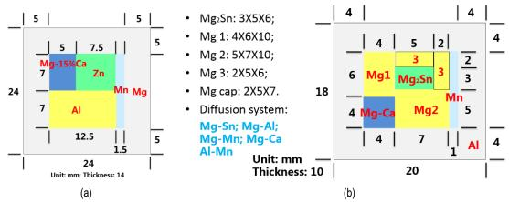
Figure III-120: Design of solid diffusion multiple: (a) the original design using a Mg cartridge; and (b) the updated design using an Al cartridge.
