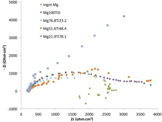
Figure III-113: Electrochemical impedance spectroscopies for the ingot pure Mg and magnetron-sputtered MgTi alloys in saturated  $Mg(OH)_2 + 0.1$  wt % NaCl solution.
