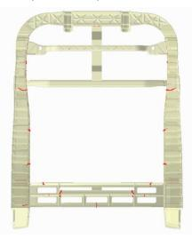
Figure IV-48: Visualization of weld lines in the back section of the complex part.
