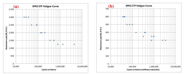
Figure V-39: Fatigue curves for pretreated Mg AM60B to Al6013 SPR joints for shear tension joints (a) and cross tension joints (b).
