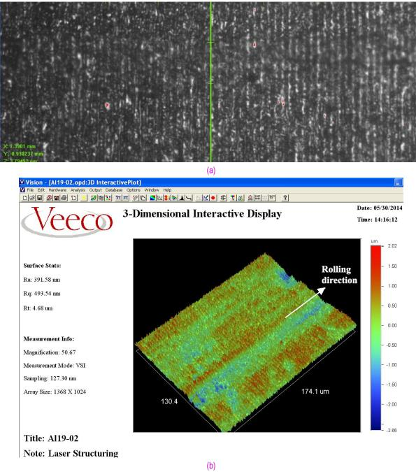
Figure V-68: Profilometry data for a laser-structured AI specimen: (a) optical micrograph showing laser-induced striations (the rolling direction is perpendicular to the laser-induced striations) and (b) profilometry data also showing laser-induced striations perpendicular to the rolling direction.
