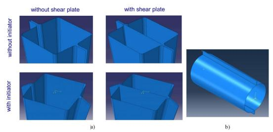
Figure IV-66: Compression molded 2-3 piece crush can concepts: (a) Hat section geometries, (b) Conical section geometries.
