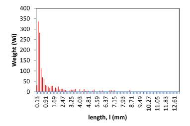
Figure IV-37: ASPN fiber length distribution for sample produced with high screw RPMs.
