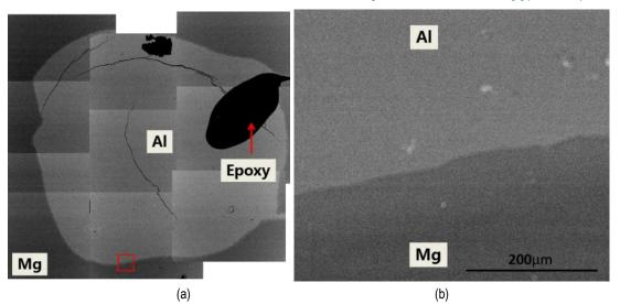
Figure III-131: BSE image of the Mg-Al diffusion multiple heat treated at 450°C for 8 hours: (a) the whole region; and (b) local region labeled by red square in Figure III-131a. The image of Figure III-131a is a combination of several images since the SEM could not take a picture of the whole region at one time.
