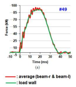
Figure IV-53: Impact force vs. time comparing discrete measurements from load cells with calculated force.
