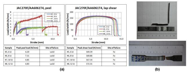
Figure V-78: Mechanical testing data for JAC270F (uncoated)/AA6061-T4 welds: (a) test data, (b) tested samples.
