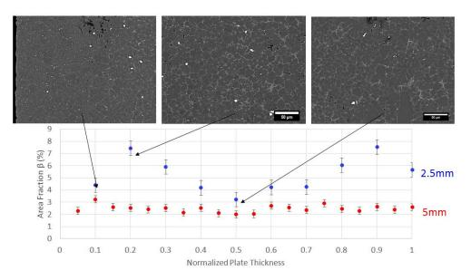
Figure III-48: A comparison of the distribution of  $\beta$ -Mg<sub>17</sub>Al<sub>12</sub> in as-cast AM70 2.5 and 5 mm plates. The  $\beta$ -Mg<sub>17</sub>Al<sub>12</sub> fraction is higher in the 2.5mm plate than the 5mm plate, and there is a peak just below the surface.
