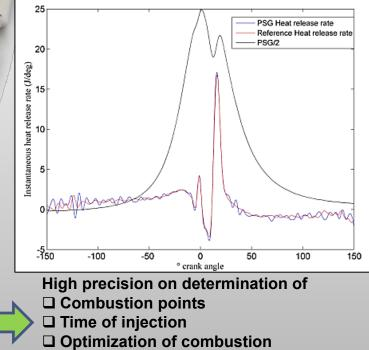
Closed-loop control on combustion
