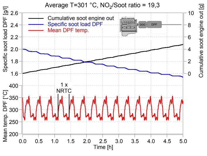
Passive regeneration works well for lead variant over NRTC
