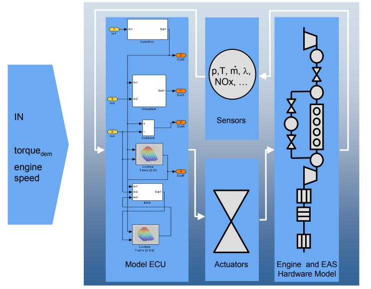
OUT torque NOx, soot, (HC, CO), temperatures, heat to coolant, BSFC
