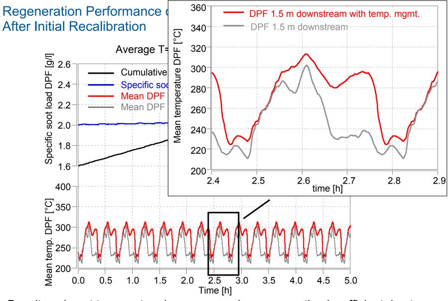
Despite exhaust temperature increase passive regeneration insufficient due to increase in engine-out emission
