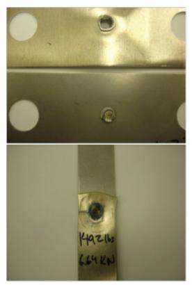
**Figure 6.** Weld button pullout failure mode observed in FBJ of AA 5754 to DP 980.
