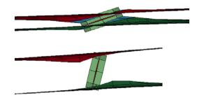
**Figure 9.** Lap-shear test simulation for large spot weld diameter.
