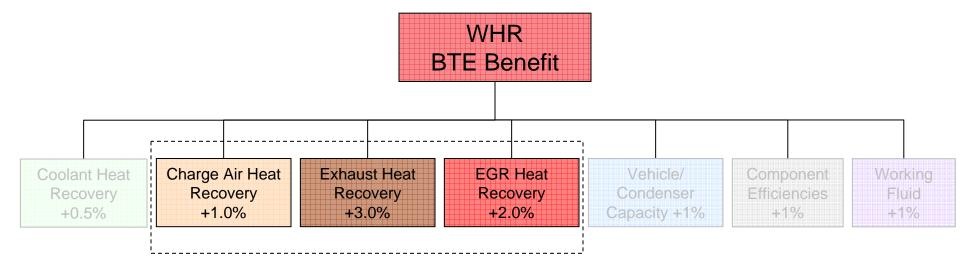
Next generation development will target the highest-return recovery opportunities – EGR, Exhaust and Charge Air – the hottest waste heat streams on the engine
