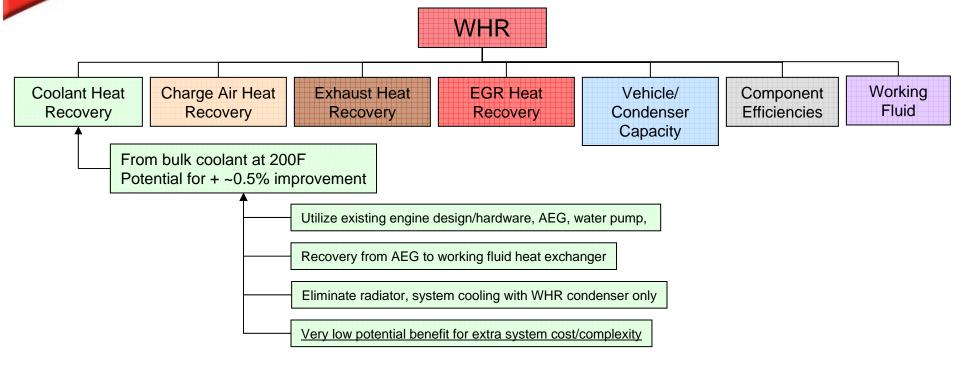
The potential recovery benefit from bulk coolant flow represents only what may be accomplished with existing architecture (AEG or non-boiling, water-based cooling).
