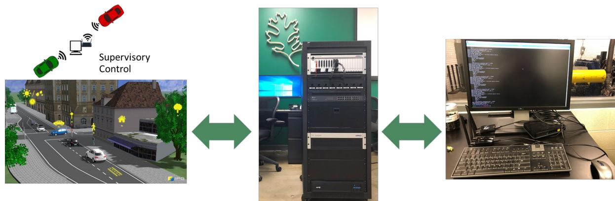
Figure IV.1.2.5 HIL testing of the V2V test in the IPG Carmaker environment.
