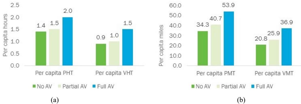
Figure I.3.5.2 Changes in (a) PMT and VMT and (b) PHT and VHT per capita by AV ownership for scenario C
