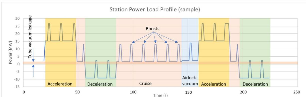
**Figure 8: Typical Load Profile for a Single Passenger Hyperloop Station.** Note: The station modeled here assumes the boosts to launch the pods and the boosts required to maintain the speed of the pods are distributed from the nearest station with infrastructure provided to the location of the boost along the route. The on-board pod batteries were assumed to be sufficient for smaller loads like passenger comfort, but not for the larger power requirements of pod acceleration and boosting.
