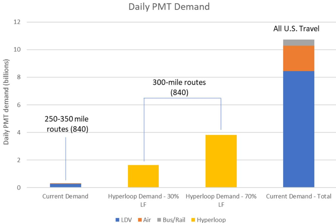
**Figure 19: Estimated daily PMT demand from 840 city pairs spaced between 250 and 350 miles apart, compared to 840 hyperloop systems operating 12 hours per day with 30-passenger pods and 2-minute launch intervals. Source for Current Demand and All U.S. Travel: National Household Travel Survey<sup>81,84</sup> Source for Hyperloop Demand: Current analysis.**
