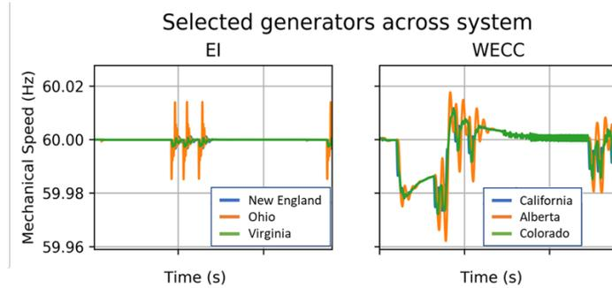
**Figure 9: System-Wide Grid Effects of Hyperloop. Shows the rotational speed of selected generators, which corresponds to the grid AC system frequency.**
