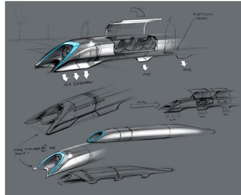
**Figure 2. Initial SpaceX Concept for Hyperloop Pod (SpaceX, 2013)**
