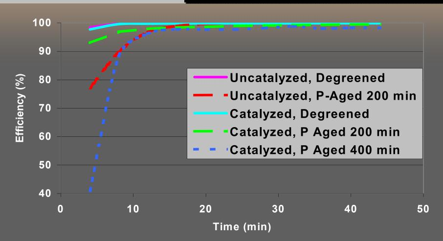
> Phosphorus aging decreases the filtration efficiency of diesel particulate filters
