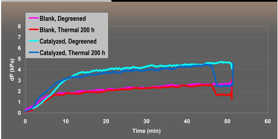
> Thermal aging of 200 hours has only a minor impact on pressure drop
