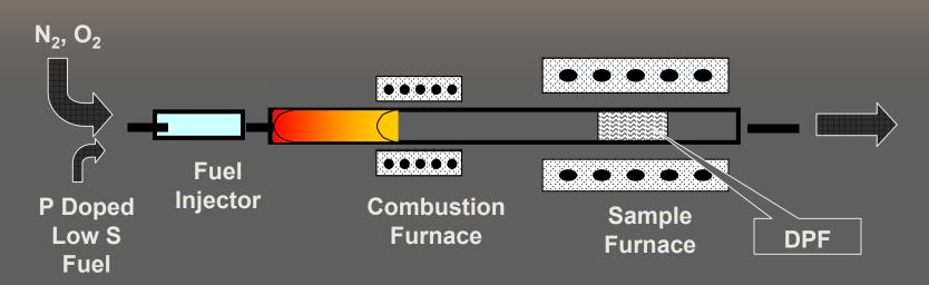
**Phosphorus (P) source:** 1% (TCP) Tri-Cresyl Phosphate [(4-CH<sub>3</sub>C<sub>6</sub>H<sub>4</sub>O)<sub>3</sub>PO]
