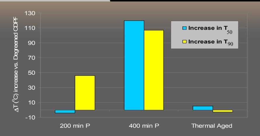
Phosphorus (P) impacts soot regeneration temperature profile more than thermal aging
