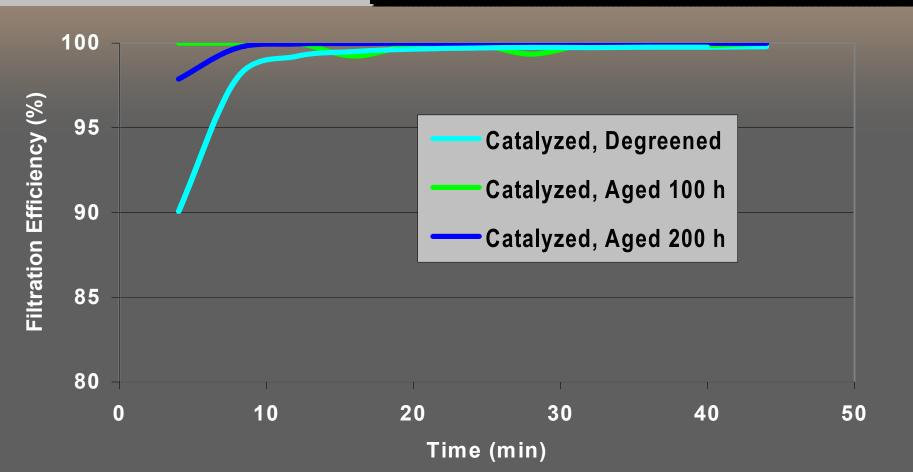
> Thermal aging of 200 hours has a minor impact on filtration efficiency
