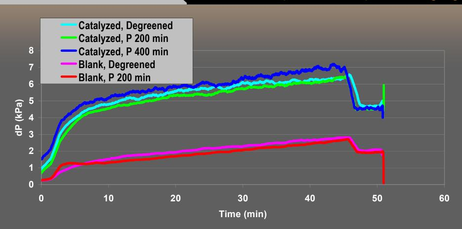
> Chemical aging by phosphorus has only a minor impact on pressure drop
