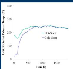
Test-to-test variability in NOx emissions as a result of temperature dependence of urea SCR
