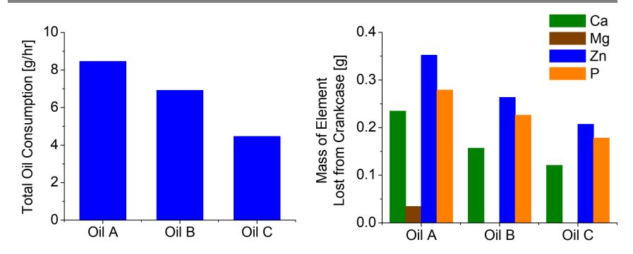
Fewer additive metals are lost from the crankcase for less volatile/higher viscosity oils
