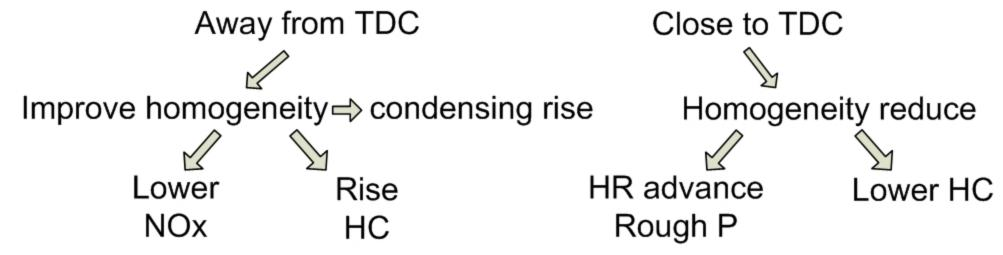
3. Minimum early injection for sufficient mixing but reduced condensing and adaptive combustion control is the key.
