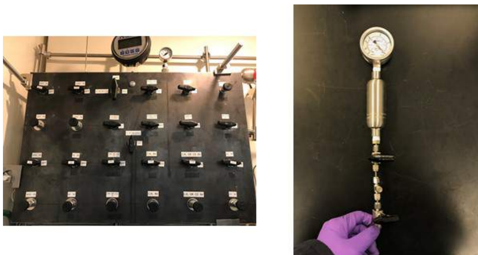
Figure II.3.G.8 Custom gas manifold control plate (left) is comprised of a series of needle and ball valves, and monitored using the digital pressure gauge ( \pm .1 torr). A typical sample cylinder containing the desired mixture allows for the direct sampling of the gas without contaminating the bulk mixture (right)
