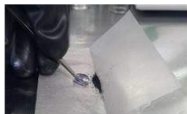
Laminate powder scraped from electrode in glovebox
