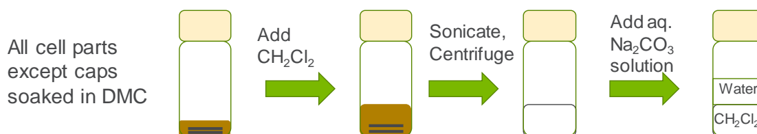
Figure II.1.A.50 Schematic of electrolyte extraction steps
