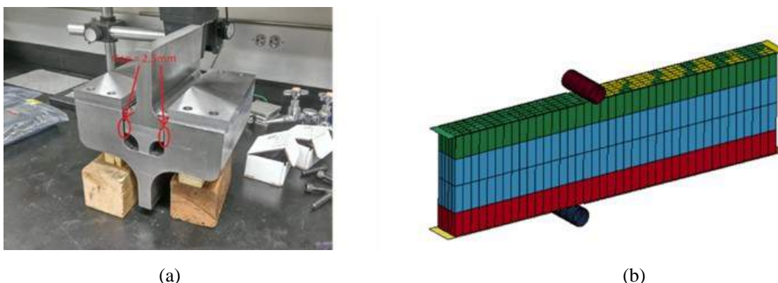
Figure I.3.D.8 Shear test. (a) experimental setup, and (b) simulation model
