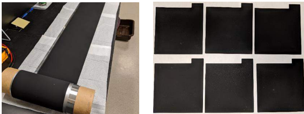
Figure II.4.E.9 Roll of NC-9604 on an 8-inch-wide Al foil. 10 x 10 cm wide defect free electrodes were punched out of the roll
