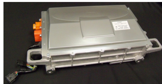
2012 Nissan LEAF® 6.6 kW OBC: 0.41kW/kg, 0.66kW/L
