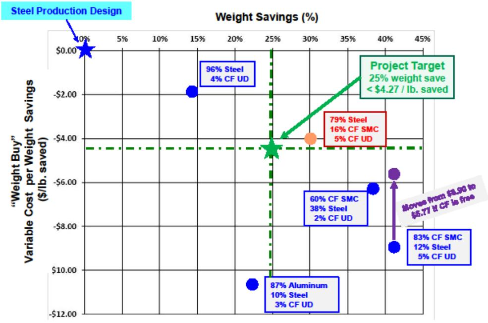
Figure 3: Weight savings and cost for various alternative designs and material compositions [11]
