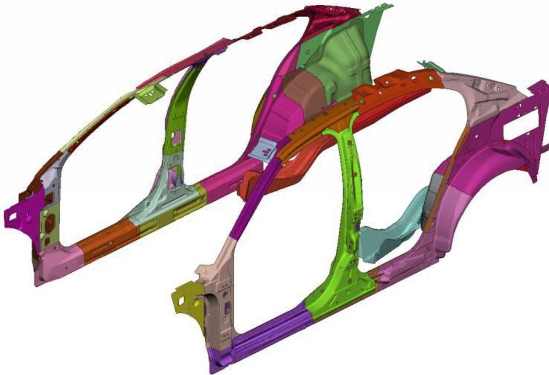
Figure 2: Side structure assembly [6]
