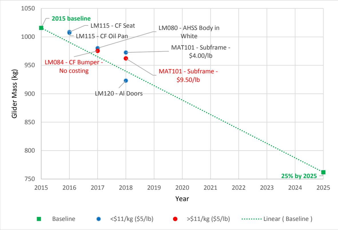
Figure 1: Chart showing cumulative mass reduction as a function of year for selected component demonstration projects that met the DOE cost target. Certain projects that did not perform a cost analysis or did not meet the cost targets are shown in red for reference but are not included in the cumulative mass reduction calculations.
