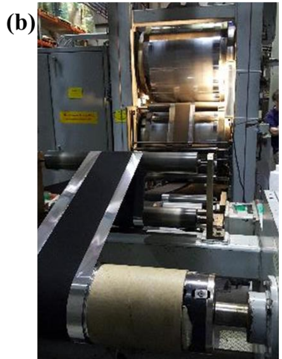
Figure: (a) PPG binder scale up. (b) Calendaring. (c) Shelf life stability test results. Mixing and coating done at Coulometrics.
