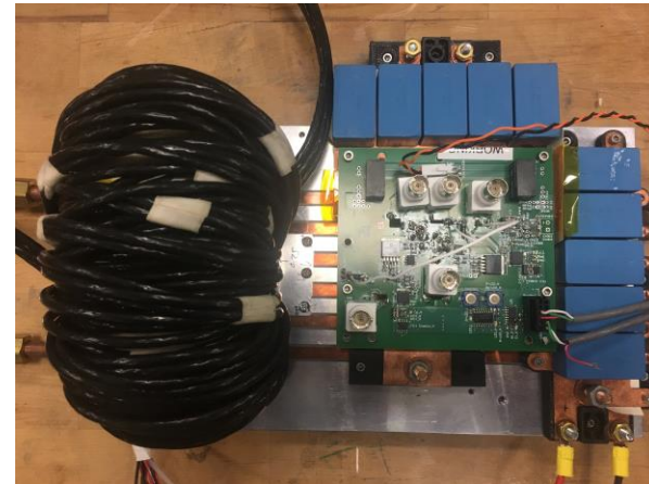
Secondary side dc-dc converter assembled using ORNL packaged WBG phase leg module
