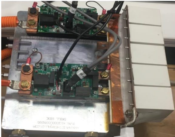
Primary side SiC inverter assembled for 85 kHz operation
