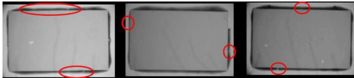
SAM image of Pressure Sintering (10MPa) of Supplier A Sinter Paste after 500 Thermal Cycles – small cracks identified at edges, not under device
