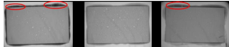
SAM image of Pressure-less Sintering of Supplier B Sinter Paste after 500 Thermal Cycles – similar small cracks identified at edges however, none under device
