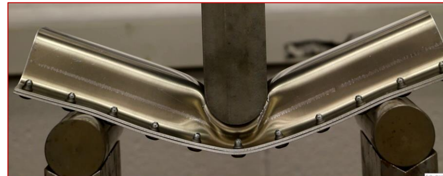
7055 Specimen: Deformation at 69mm of ram stroke
