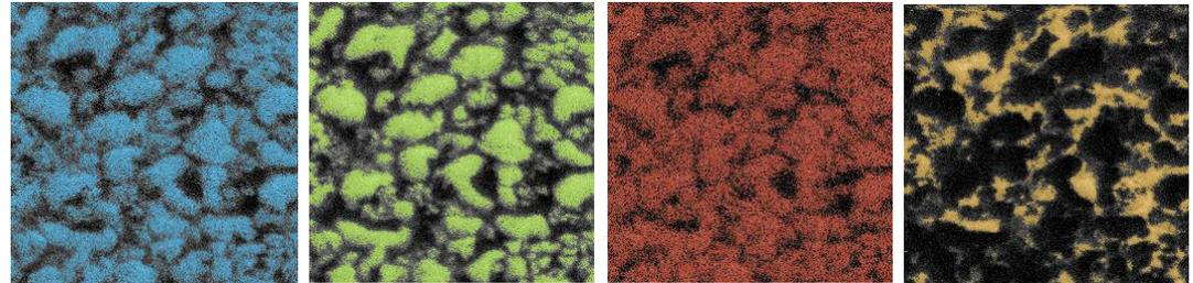
Post-Sputter Elemental Maps of Co (blue), O (lime), F (red), and C (yellow) of a 4.5V LCO Cell Cycled at .7C
