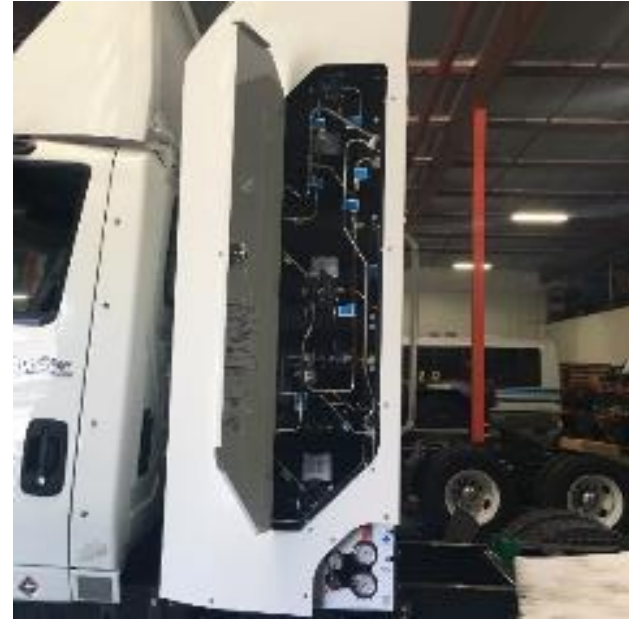
Truck shown with Hydrogen fuel tanks installed behind cab (truck shown is identical to Air Liquide trucks).
