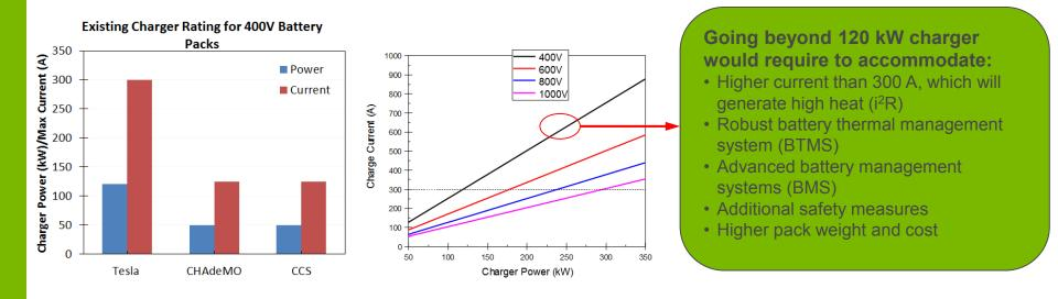
A high voltage pack will lower the maximum charging current, but require additional design and safety modifications.
