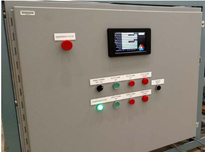
Flame Supervision Control Cabinet (NFPA 86)
