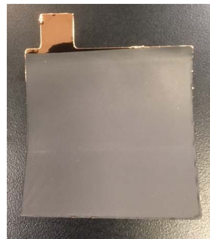
Composite current collector roll and electrode for use in a pouch cell build.
