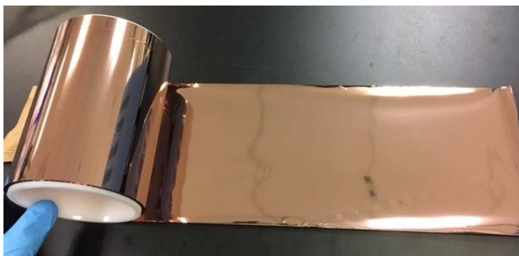
Composite current collector roll and electrode for use in a pouch cell build.
