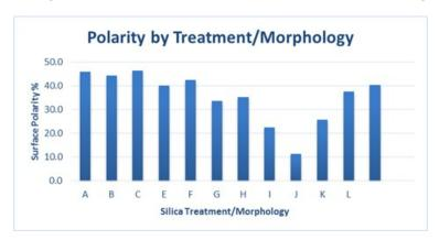
Reduced Payne Effect by Reducing Surface Energy Lower G' at low strain, lower filler-filler interaction
