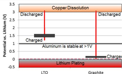
LTO and graphite potential vs. lithium in reference to lithium plating, aluminum stability and copper dissolution. The red line is the total potential range (including first charge and complete discharge) while the black rectangle is the typical operating potential. LTO operates in a potential range far from lithium plating and where aluminum is stable providing cycle life and safety advantage plus indefinite 0V storage capability when coated on aluminum substrate.
