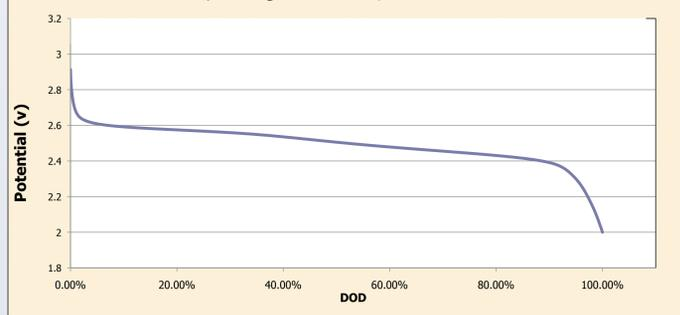
Discharge curve for a typical LTO/LMO cell demonstrating a relatively flat profile
