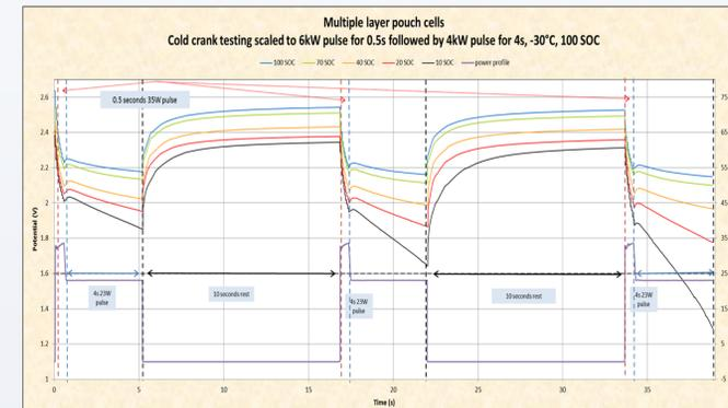
Cold crank testing was performed on multi-layer pouch cells using LMO as the positive electrode and LTO as the negative electrode.
