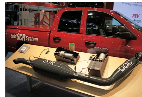
FEV solid SCR system: Ammonium carbamate
