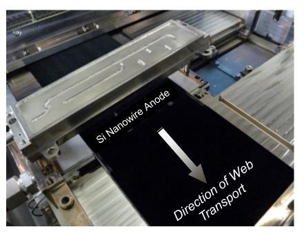
During Q1 2016, Amprius tested a first of its kind pilot line tool for roll-to-roll production of double-sided, rooted silicon nanowire anodes
