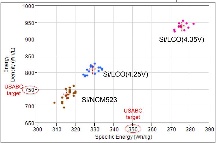
•Cathode energy density and specific energy has to be higher than that of NMC523 – minimum 180 mAh/g
